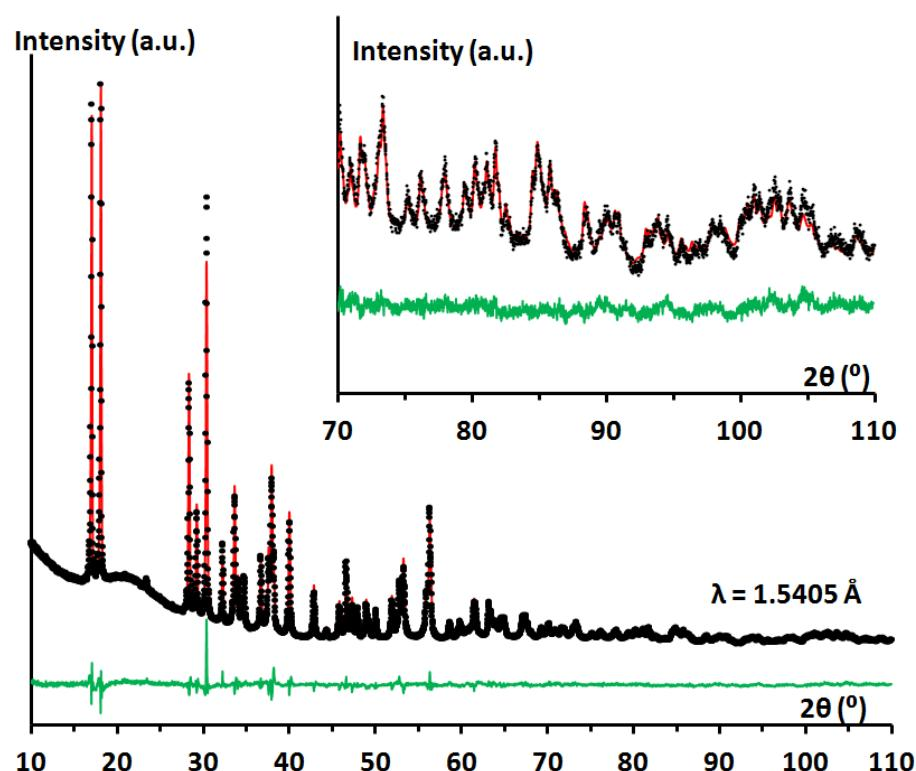
The Rietveld fit in the  $\text{Na}_2\text{CuF}_4$ -type structure is depicted by a red line. Green lines depict the difference between the fit and experimental points.
