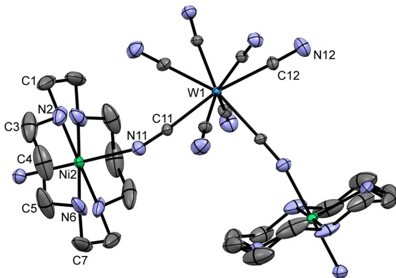
**Fig. S1** Structure of  $1A \cdot 16H_2O$  with atom numbering; thermal ellipsoids at 50% probability; water molecules and hydrogen atoms omitted for clarity.
