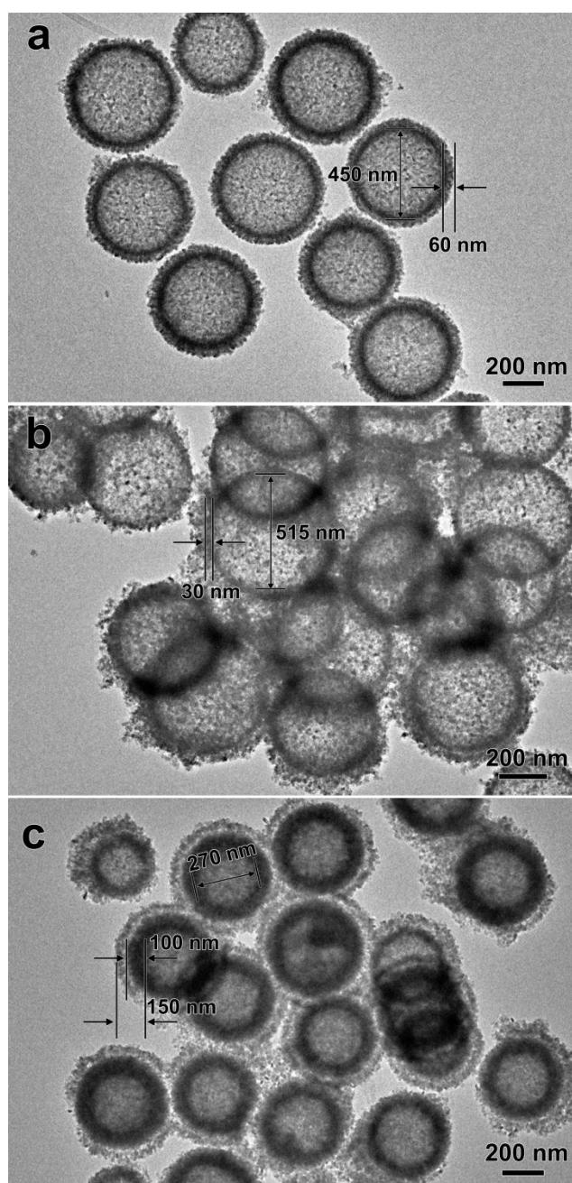
**Electronic Supplementary Information, Figure S2.** TEM images of  $\text{YVO}_4:\text{Eu}^{3+}$  hollow spheres (a) S5, (b) S6
