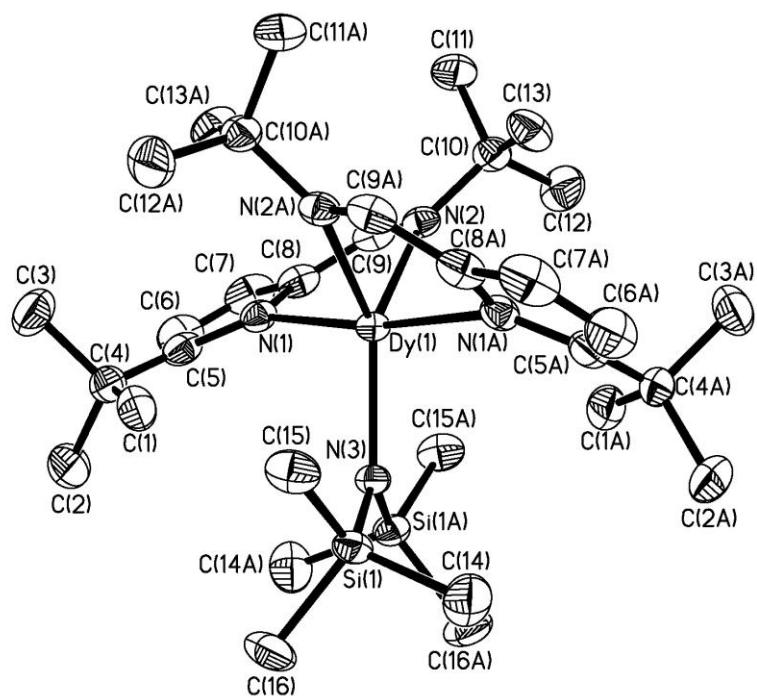
**Figure 6.** Molecular structure of the compound **4b**, hydrogen atoms are omitted for clarity. Selected bond lengths ( $\text{\AA}$ ) and angles ( $^{\circ}$ ): Dy(1)-N(1) 2.421(2), Dy(1)-N(2) 2.4136(19), Dy(1)-N(3) 2.232(3), C(9)-N(2) 1.302(3), N(3)-Dy(1)-N(1) 94.14(4), N(3)-Dy(1)-N(2) 131.93(5), N(1)-Dy(1)-N(2) 73.12(7), N(1)-Dy(1)-N(1A) 171.72(9), N(1)-Dy(1)-N(2A) 101.19(7), N(2)-Dy(1)-N(2A) 96.13(9), N(2)-C(9)-C(8) 124.6(2).
