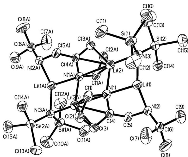
**Figure 9.** Molecular structure of the compound **5**, hydrogen atoms are omitted for clarity. Selected bond lengths ( $\text{\AA}$ ) and angles ( $^{\circ}$ ): Li(1)-N(1) 2.057(4), Li(2)-N(1A) 2.693(4), Li(1)-N(2) 2.057(4), Li(2)-C(1A) 2.536(5), Li(1)-N(3) 1.960(4), Li(2)-C(2A) 2.332(4), Li(2)-N(1) 2.134(4), Li(2)-C(3A) 2.339(4), Li(2)-N(3) 2.064(4), Li(2)-C(4A) 2.553(4), C(5)-N(2) 1.484(3), N(2)-C(5)-C(4) 111.59(18).
