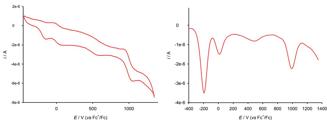
**Figure S1.** CV (left) and OSWV (right) of mononuclear complex **11** ( $c = 5 \cdot 10^{-4}\text{ M}$ ) in  $\text{CH}_2\text{Cl}_2/\text{CH}_3\text{CN}$  (1:1) with 0.1 M of TBAHP as supporting electrolyte.
