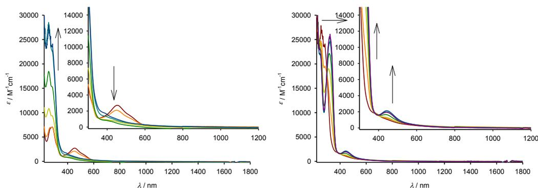
**Figure S7.** Evolution of UV-Vis-NIR spectra during the course of the oxidation of complex **19** ( $c = 5 \times 10^{-4}$  M) in  $\text{CH}_2\text{Cl}_2/\text{CH}_3\text{CN}$  (1:1) with  $[(\text{nBu})_4\text{N}]\text{PF}_6$  (0.15 M) as supporting electrolyte when: a)  $0 < n < 2$  (left), or b)  $2 < n < 4$  (right) electrons are removed. Arrows indicate absorptions that increase or decrease during the experiment.
