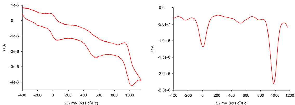
**Figure S2.** CV (left) and OSWV (right) of binuclear complex **19** ( $c = 5 \times 10^{-4} \text{ M}$ ) in  $\text{CH}_2\text{Cl}_2/\text{CH}_3\text{CN}$  (1:1) with 0.1 M of TBAHP as supporting electrolyte.
