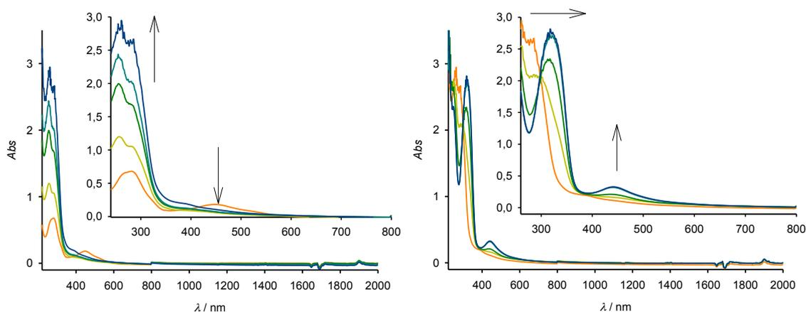
**Figure S6.** Evolution of UV-Vis-NIR spectra during the course of the oxidation of complex **13** ( $c = 5 \times 10^{-4}$  M) in  $\text{CH}_2\text{Cl}_2/\text{CH}_3\text{CN}$  (1:1) with  $[(\text{nBu})_4\text{N}]\text{PF}_6$  (0.15 M) as supporting electrolyte when: a)  $0 < n < 2$  (left), or b)  $2 < n < 4$  (right) electrons are removed. Arrows indicate absorptions that increase or decrease during the experiment.
