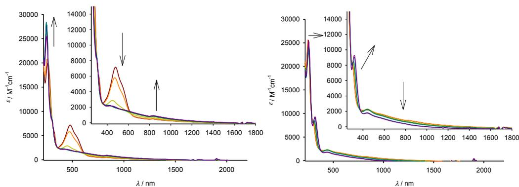
**Figure S5.** Evolution of UV-Vis-NIR spectra during the course of the oxidation of complex **12** ( $c = 5 \times 10^{-4}$  M) in  $\text{CH}_2\text{Cl}_2/\text{CH}_3\text{CN}$  (1:1) with  $[(\text{nBu})_4\text{N}]\text{PF}_6$  (0.15 M) as supporting electrolyte when: a)  $0 < n < 2$  (left), or b)  $2 < n < 4$  (right) electrons are removed. Arrows indicate absorptions that increase or decrease during the experiment.
