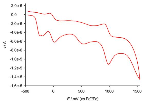
**Figure S4.** CV (left) of binuclear complex **12** ( $c = 5 \cdot 10^{-4} \text{ M}$ ) in  $\text{CH}_2\text{Cl}_2/\text{CH}_3\text{CN}$  (1:1) with 0.1 M of TBAHP as supporting electrolyte.
