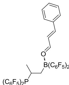
Bis(pentafluorophenyl)-2-propenylphosphane (9) (150 mg, 0.375 mmol) and bis(pentafluorophenyl)borane (130 mg, 0.375 mmol) were dissolved in *n*-pentane (5 mL) and after stirring for five min the reaction mixture turned cloudy. Cinnamic aldehyde (50.0 mg, 0.375 mmol) was added to the reaction mixture which turned green-yellow and a white solid precipitated. The solid was isolated *via* filter cannula, washed with *n*-pentane (15 mL) and dried
