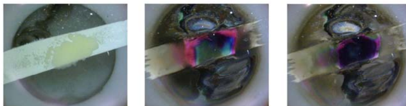
Fig. S15 Photographic image of the colour change of the solid Zn(NDC)(DPMBI) material at the transparent ITO-Quartz working electrode. The image at far left shows the neutral material (0 V) and the two images to the right show the colour changes as a potential of -2.20 V is applied to the cell.
