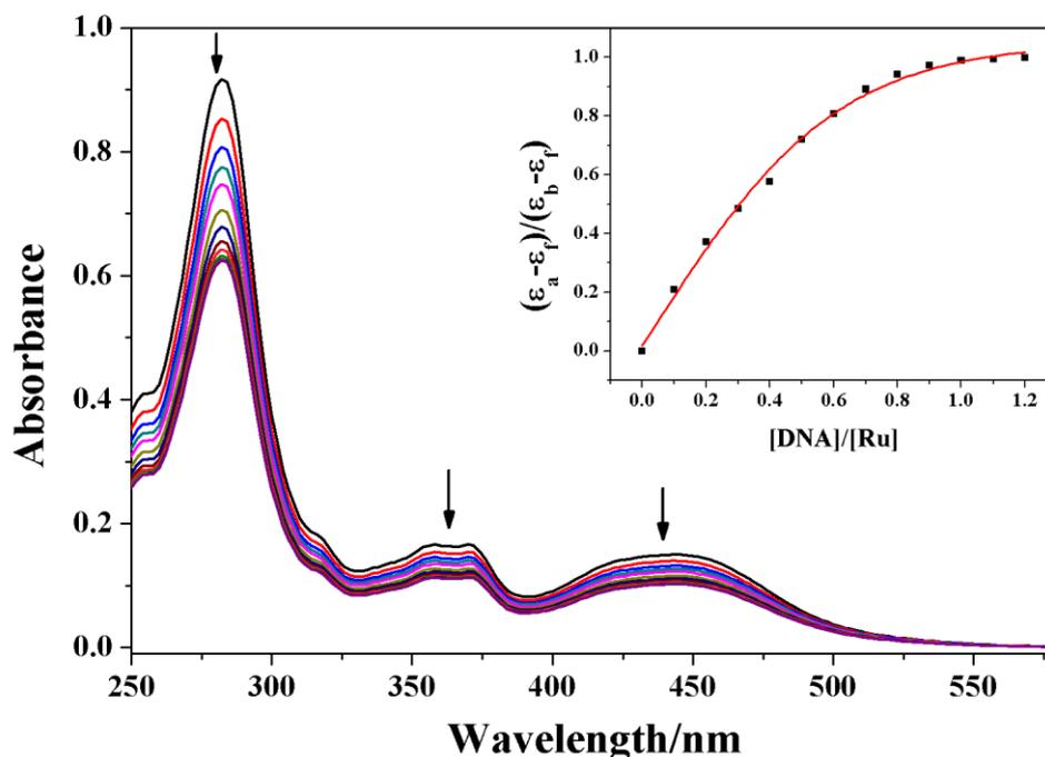
**Fig. S2** Absorption spectra of  $[\text{Ru}(\text{bpy})_2\text{dppz}]^{2+}$  (10  $\mu\text{M}$ ) in the presence of 22AG (0–12  $\mu\text{M}$ ) in  $\text{K}^+$  buffer (10 mM Tris, 100 mM KCl, pH 7.0). Inset: plot of  $(\varepsilon_a - \varepsilon_f)/(\varepsilon_b - \varepsilon_f)$  vs.  $[\text{DNA}]$  (using absorbance at 450 nm).
