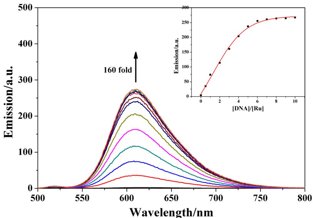
**Fig. S3** Fluorescence spectra of [Ru(bpy)<sub>2</sub>dppz-idzo]<sup>2+</sup> (2.5 μM) upon titration with calf thymus DNA (CT-DNA) in buffer solution containing 10 mM Tris, 50 mM NaCl, 1 mM EDTA, pH 7.5. Inset: plot of emission intensity at 605 nm vs. [DNA]/[Ru] and the best fit for the titration of Ru(II) complex with CT-DNA.
