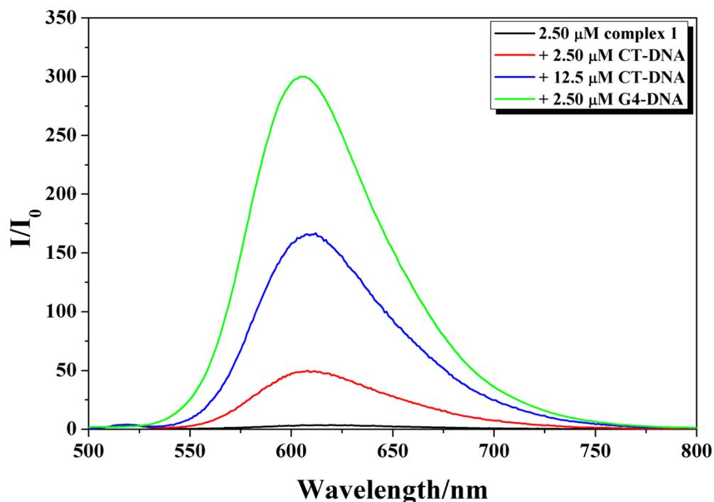
**Fig. S4** Fluorescence spectrum of complex 1 (2.5 μM) in the absence of DNAs (black line), in the presence of 2.5 μM of calf thymus DNA (red line), 12.5 μM of calf thymus DNA (blue line), and 2.5 μM of quadruplex DNA (green line).
