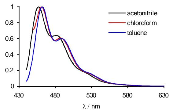
**Figure S3.** Emission spectra of **8** in different solvents ( $\text{ca.} 10^{-5}$  M) at room temperature
