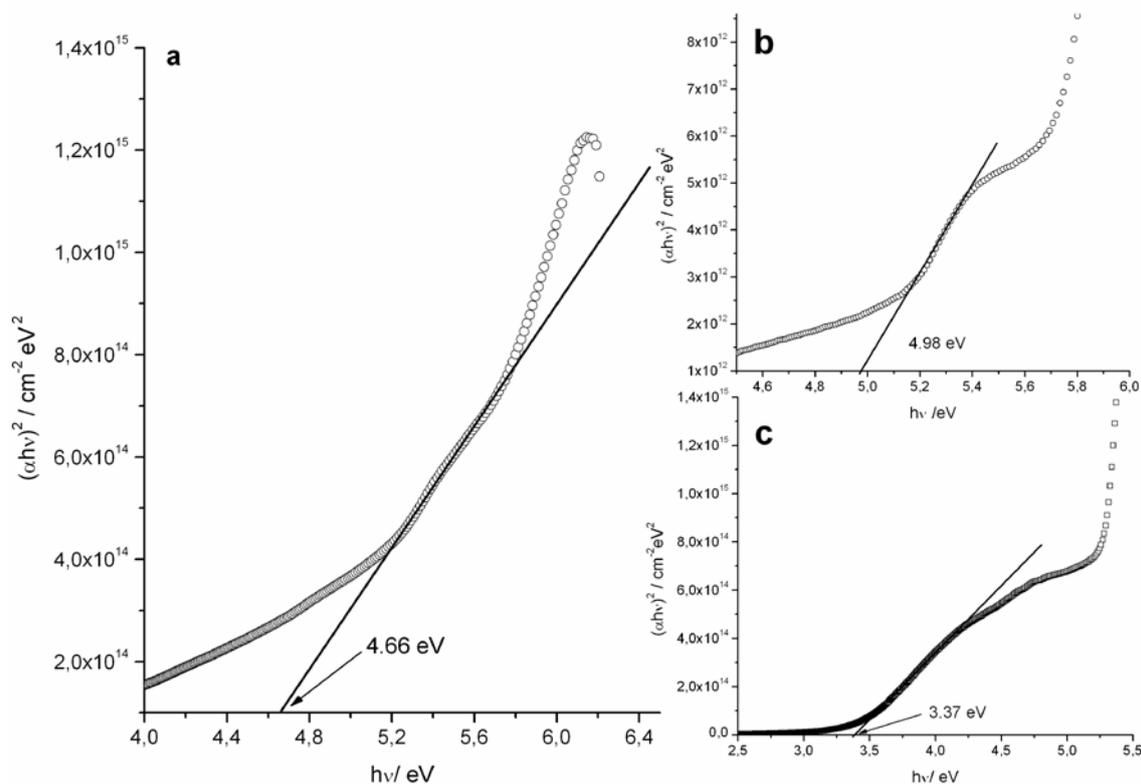
Band gap energy estimation of (a) Si-Ce<sub>2</sub>, (b) Si<sub>2</sub> and (c) CeO<sub>2</sub> nanomaterials by plotting  $(\alpha hv)^m$  of the microcrystalline materials against the photon energy ( $h\nu$ ).
