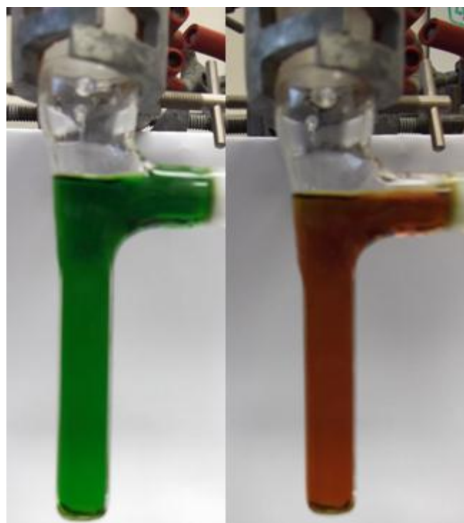
Figure S52. A significant colour change is observed upon controlled potential coulometry experiment at -1.8 V for [\text{Ni}^{\text{II}}\text{L}^{\text{Pr}}](\text{BF}_4) which resulted in the transfer (removal) of 1.1 electron equivalents. Left: before; Right: after.
