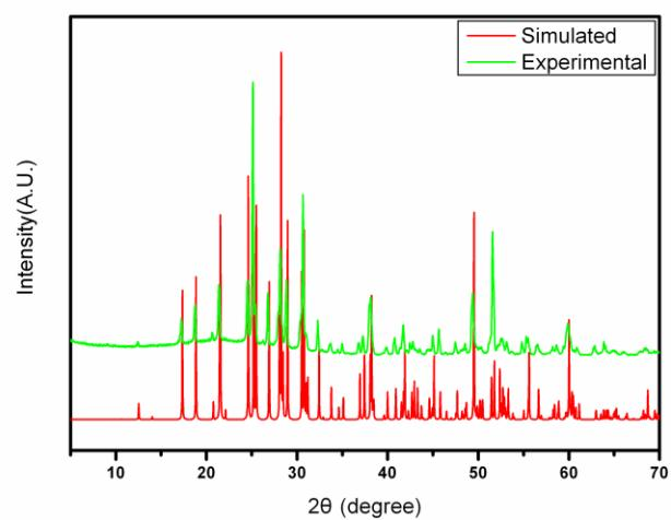
Figure S1. Experimental and simulated powder X-ray diffraction data for  $\text{Tl}(\text{VO})_2\text{O}_2(\text{IO}_3)_3$ .
