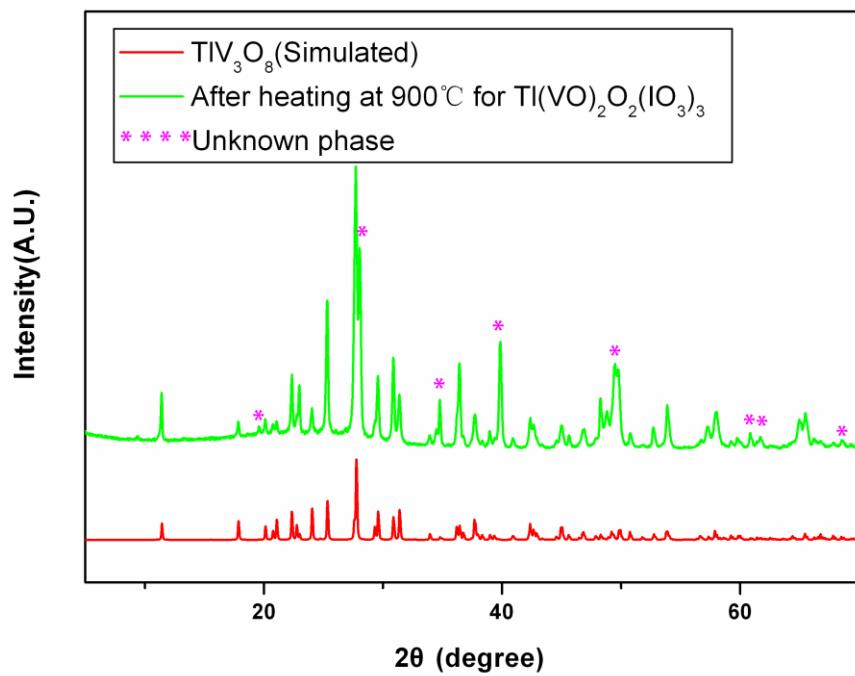
Figure S2. Powder X-ray diffraction studies for the thermal decomposition products of  $\text{Tl}(\text{VO})_2\text{O}_2(\text{IO}_3)_3$ .
