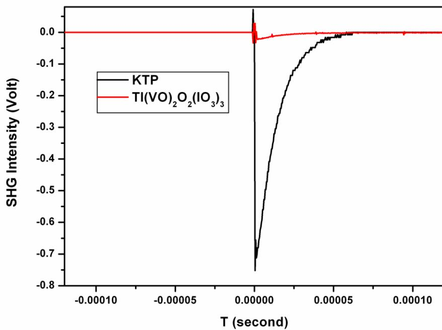
Figure S4. The measured SHG signal of  $\text{Tl}(\text{VO})_2\text{O}_2(\text{IO}_3)_3$  in the particle size range of 50-70 mesh compared with that of KTP under 1064 nm laser radiation .
