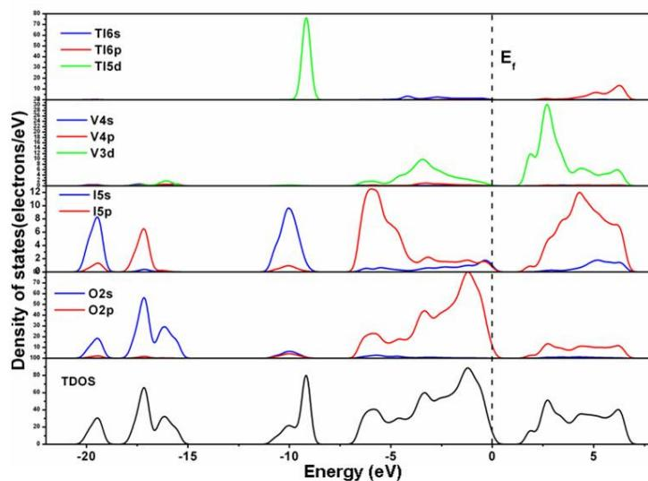
Figure S6. Electronic density of states of  $\text{Tl}(\text{VO})_2\text{O}_2(\text{IO}_3)_3$ .
