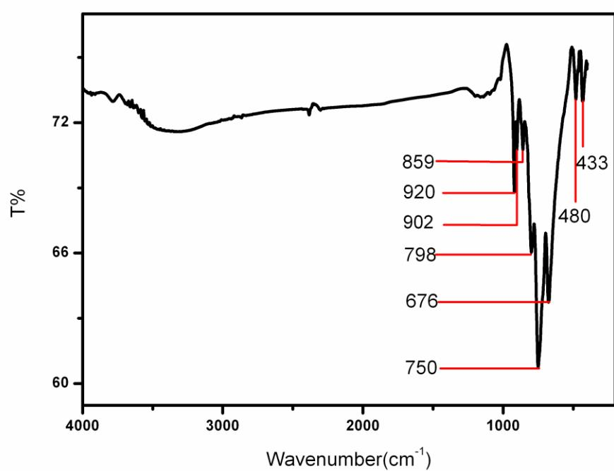
Figure S3. The infrared spectra of  $\text{Tl}(\text{VO})_2\text{O}_2(\text{IO}_3)_3$ .
