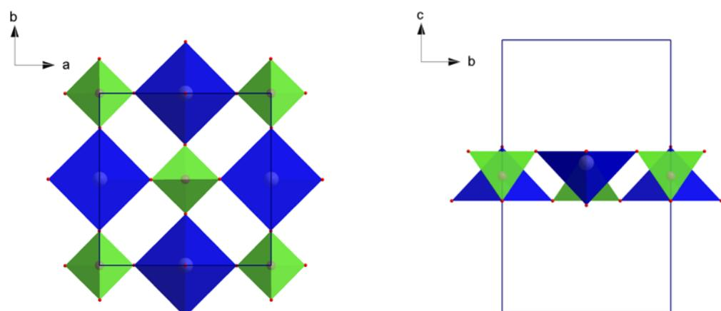
**Figure S1.** Representation of  $\alpha_1\text{-VOPO}_4$  layer isolated in a supercell. Blue square pyramids and green tetrahedra represent VO<sub>5</sub> and PO<sub>4</sub> units, respectively.
