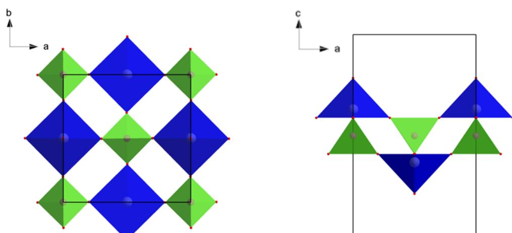
**Figure S5.** Representation of  $\alpha_2\text{-VOPO}_4$  layer isolated in a supercell. Blue square pyramids and green tetrahedra represent  $\text{VO}_5$  and  $\text{PO}_4$  units, respectively.
