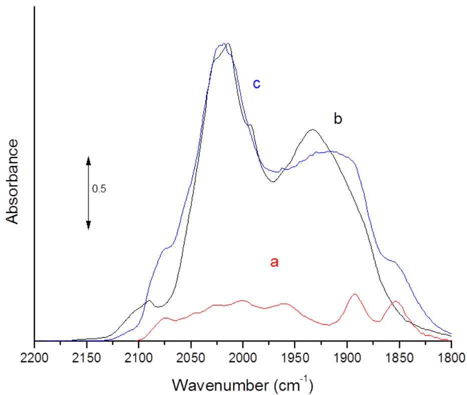
**Figure S1.** IR spectra (absorbance) in the  $\nu_{\text{CO}}$  region characterizing MgO-supported samples treated at 393 K for 1 h in flowing  $\text{H}_2$  followed by a CO pulse at 298 K: (a)  $\text{Rh}(\text{C}_2\text{H}_4)_2$ , (b)  $[\text{Os}_3(\text{CO})_{11}]^{2-}$ , (c)  $[\text{Os}_3(\text{CO})_{11}]^{2-} + \text{Rh}(\text{C}_2\text{H}_4)_2$ .
