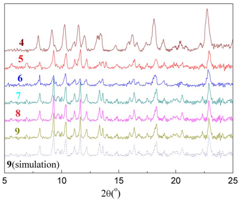
**Fig. S13** Experimental X-ray powder patterns for microcrystalline samples **4–9** and simulated pattern for **9**.
