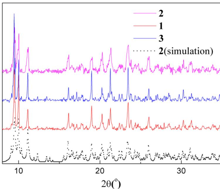
**Fig. S12** Experimental X-ray powder patterns for microcrystalline samples **1–3** and simulated pattern for **1**.
