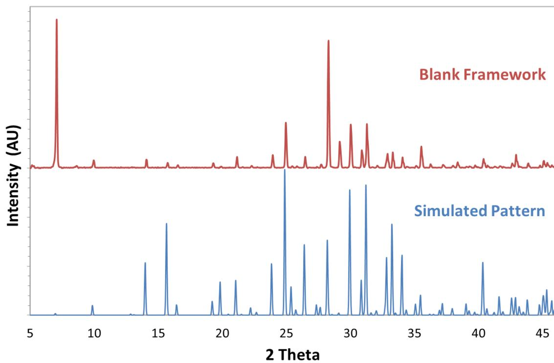
ESI Figure 1.1 – Simulated powder XRD pattern (blue line) and experimental XRD of the blank framework (red line), showing the structural integrity of the uncalcined framework
