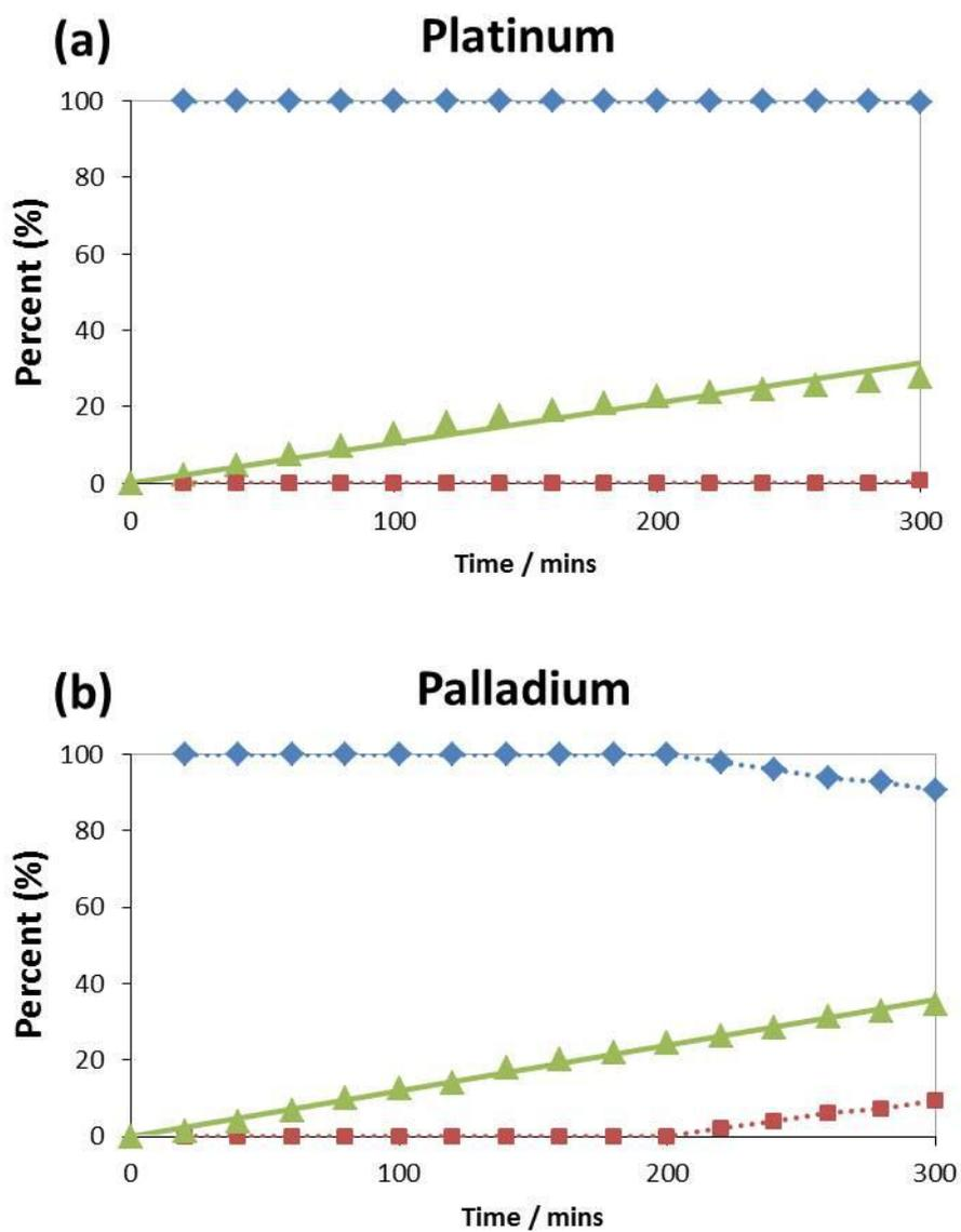
ESI Figure 3.7 - Benzyl alcohol conversion (green triangles), benzaldehyde selectivity (blue diamonds) and benzoic acid selectivity (red squares) for the platinum (a) and palladium (b) catalysts at 120 °C under 20 bar of air.
