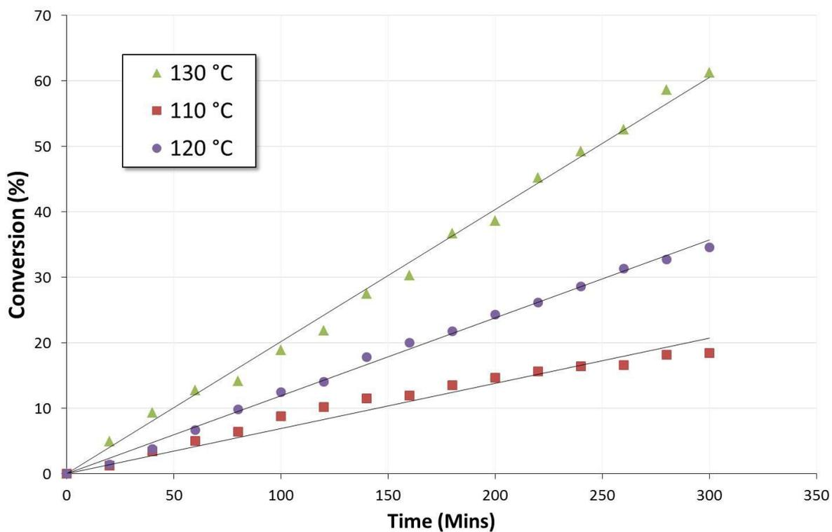
ESI Figure 3.5 - Kinetic plots for conversion of benzyl alcohol in aerobic oxidation with Pd catalyst at varying temperatures
