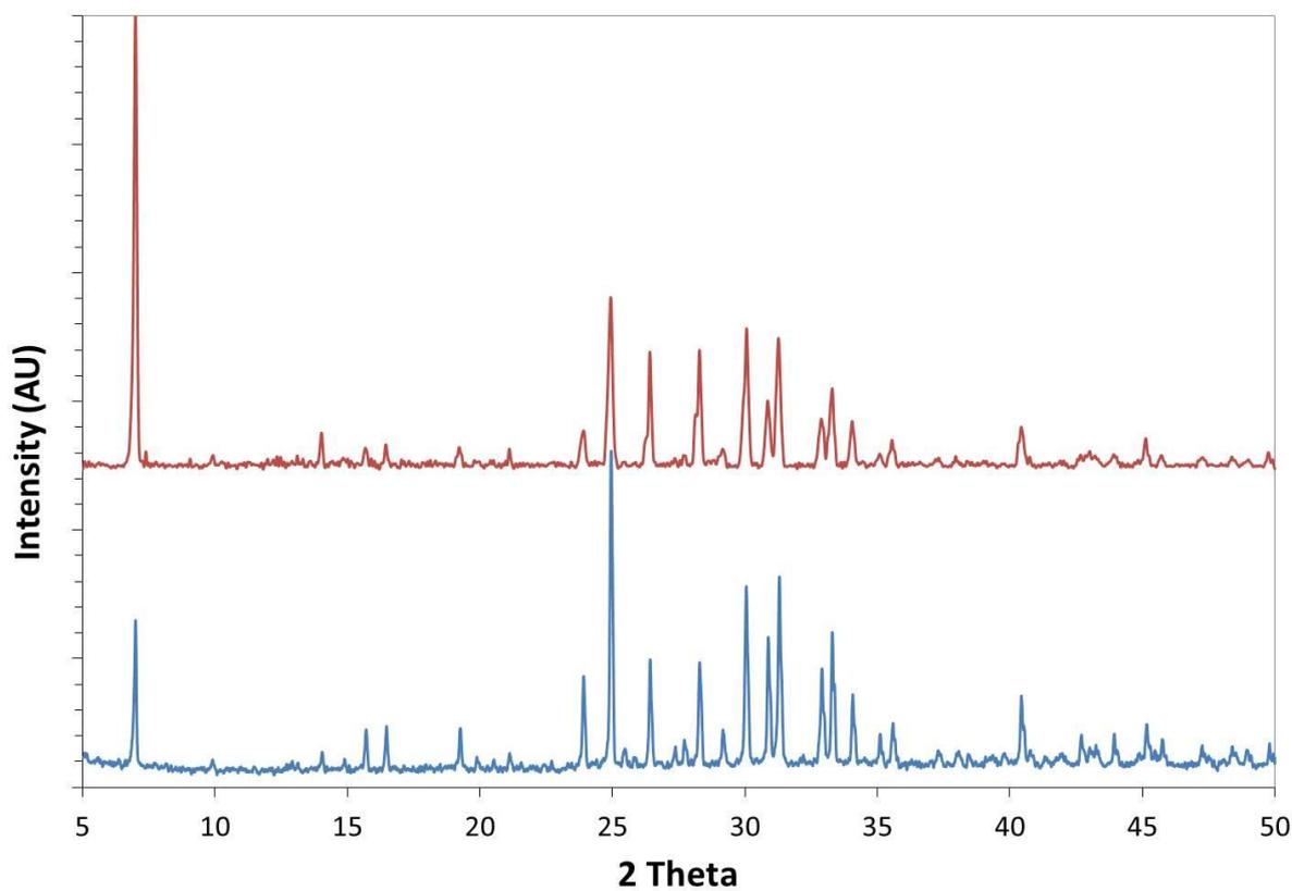
ESI Figure 2.2 – Powder XRD of calcined (blue line) and used (red line) palladium catalyst
