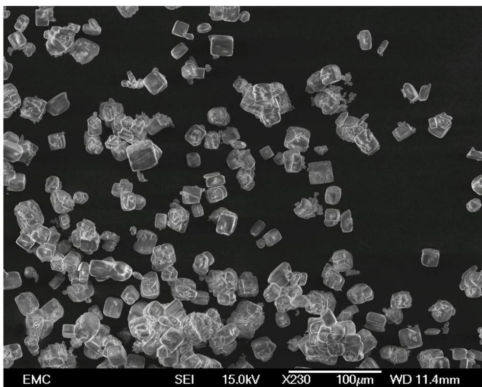
ESI Figure 5.2 – SEM Micrograph depicting the homogeneous morphology of crystals across a sample
