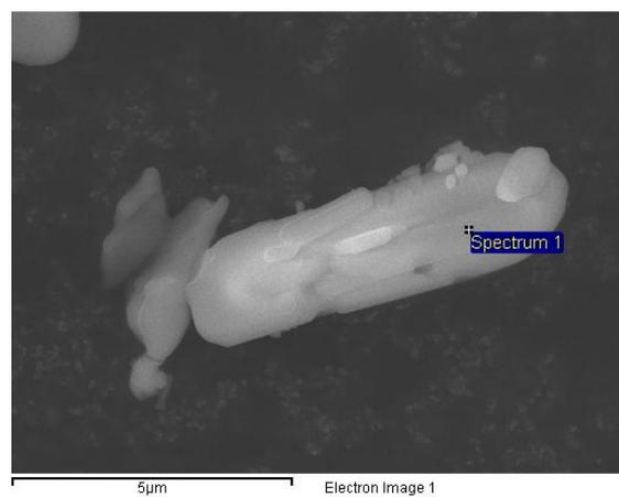
ESI Figure 6.2 – EDX spectra of calcined platinum catalyst
