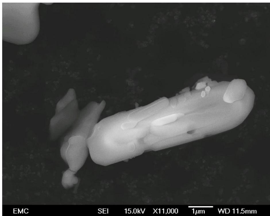
ESI Figure 5.3 – SEM Micrograph of platinum catalyst post-calcination with platinum particles visible on the surface
