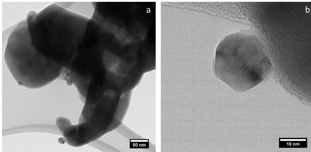
ESI Figure 7.1 - TEM image of the calcined Pd catalyst showing the presence of faceted nanocrystals.
