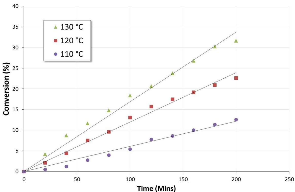
ESI Figure 3.3 - Kinetic plots for conversion of benzyl alcohol in aerobic oxidation with Pt catalyst at varying temperatures
