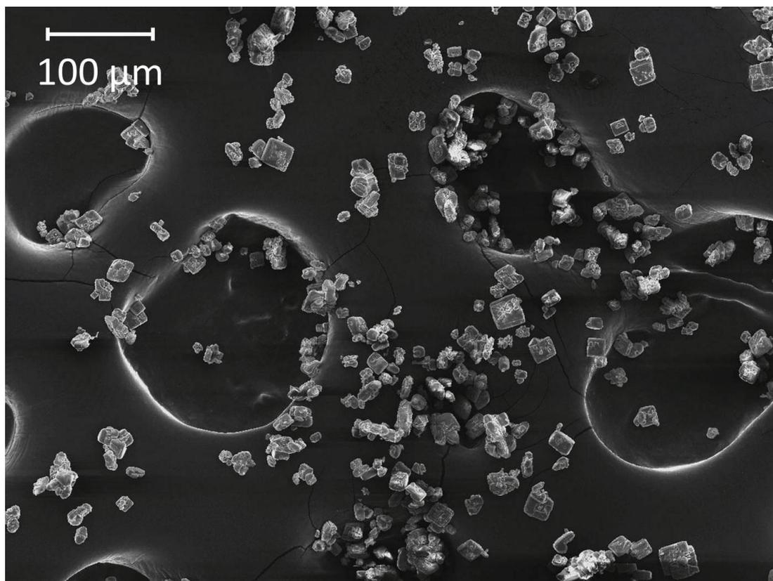
ESI Figure 5.4 – SEM Micrograph depicting the homogeneous morphology of crystals across a sample
