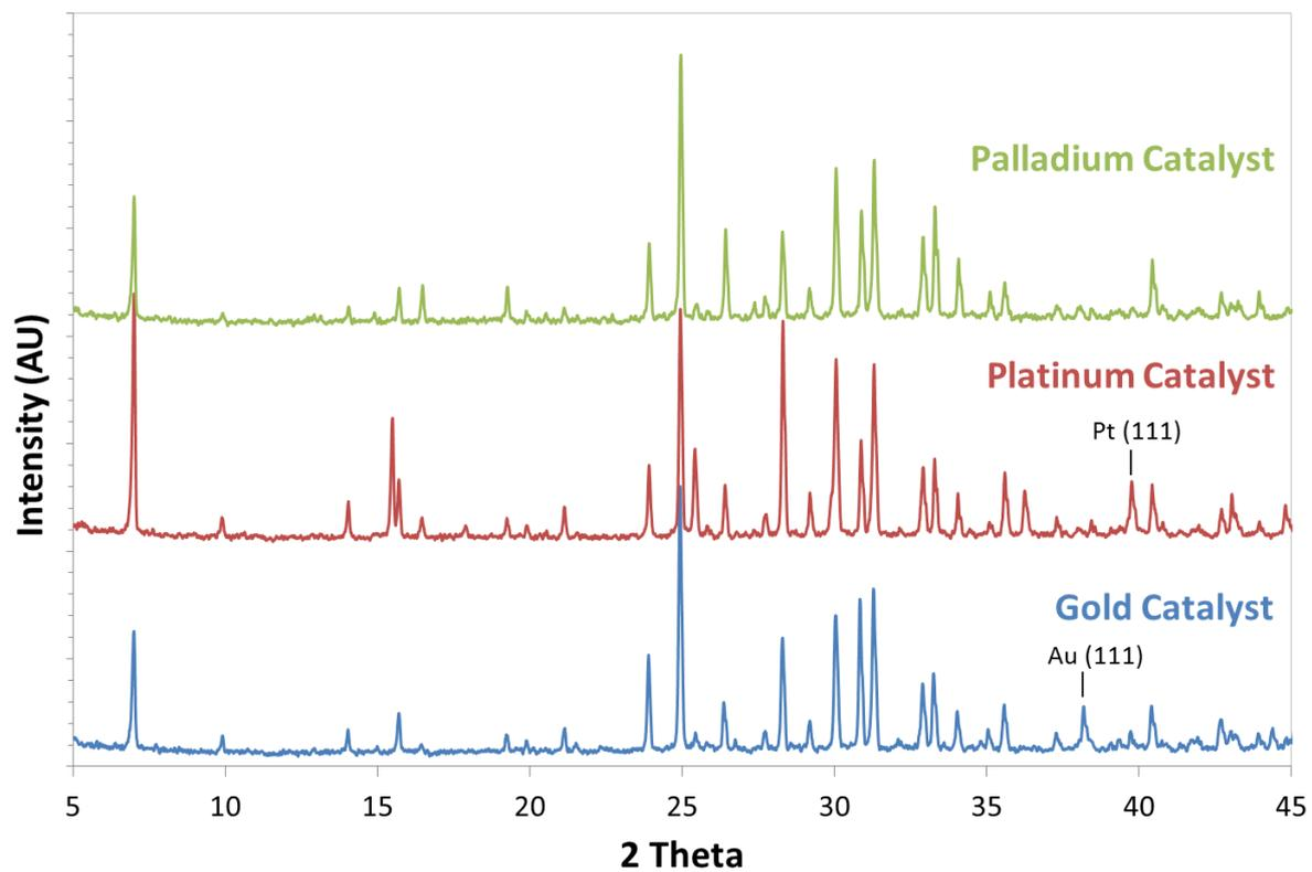
ESI Figure 1.2 Powder XRD patterns of each catalyst material calcined @ 500°C (Blue line – Au catalyst; Red line – Pt catalyst; Green line – Pd catalyst)
