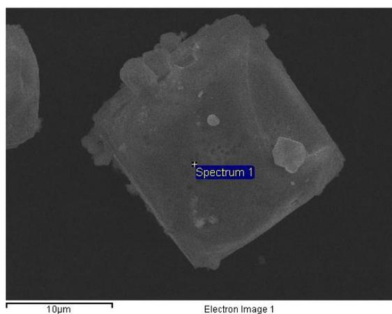
ESI Figure 6.1 - EDX Spectra of as-synthesised platinum catalyst
