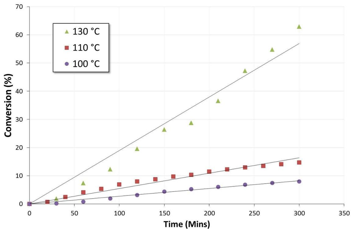
ESI Figure 3.1 - Kinetic plots for conversion of benzyl alcohol in aerobic oxidation with Au catalyst at varying temperatures
