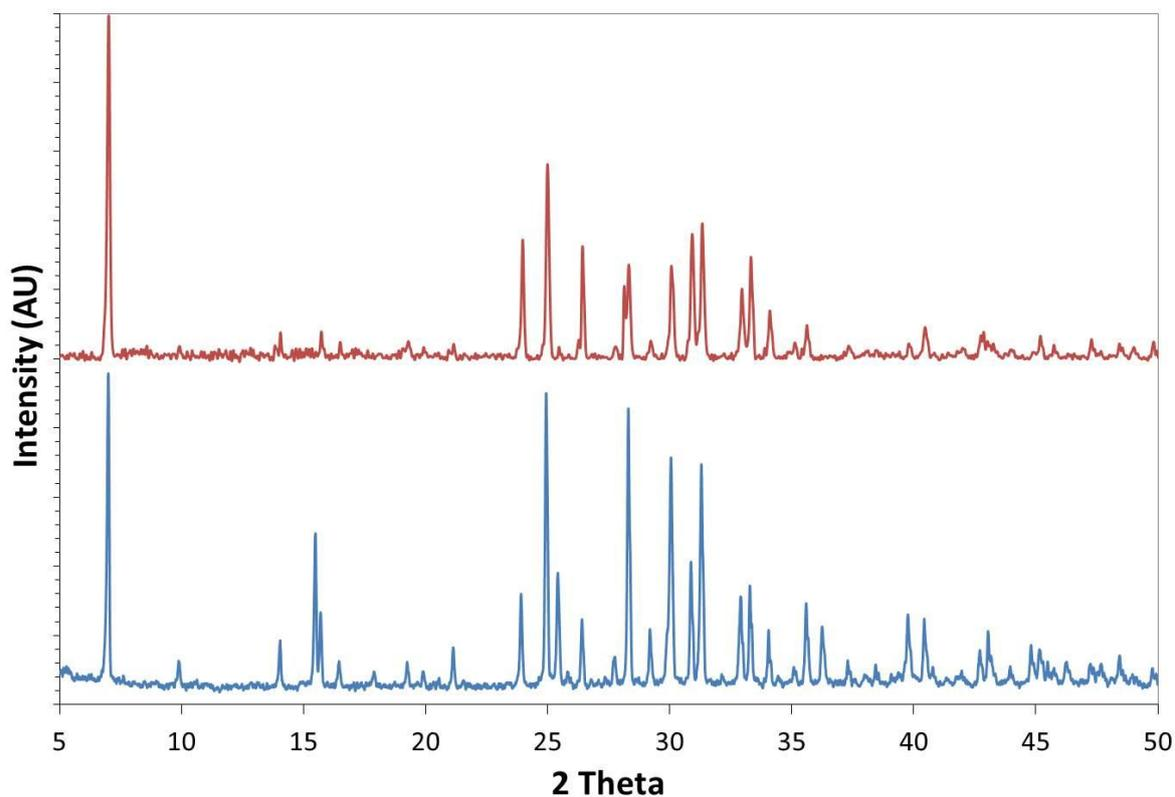
ESI Figure 2.1 – Powder XRD of calcined (blue line) and used (red line) platinum catalyst
