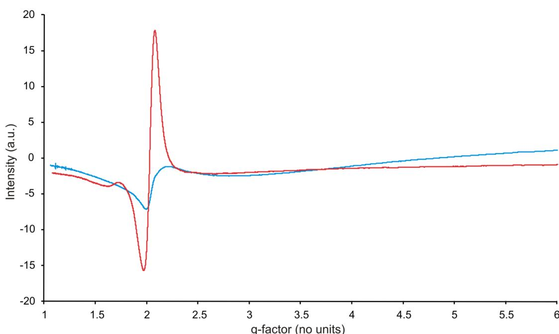
**Figure S2.** X-band (9.3896 GHz) CW EPR spectrum of a solid sample of **1** recorded at 296 K (blue) and at 15 K (red).
