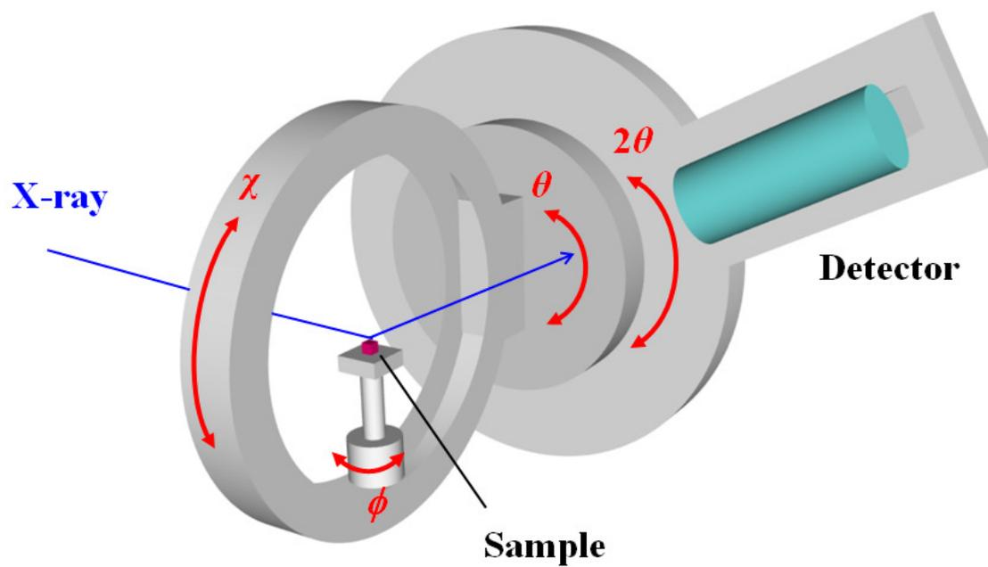
**Fig. S1** The schematic drawing of the four-circle diffractometer at beamline BL13XU for surface and interface structures, SPring-8.
