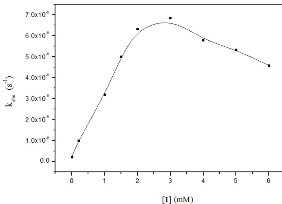
**Figure S11.** Influence of the concentration of **1** on the observed rate constant for the hydrolysis of 2.0 mM Gly-Ser at pH 5.4 and 60 °C.
