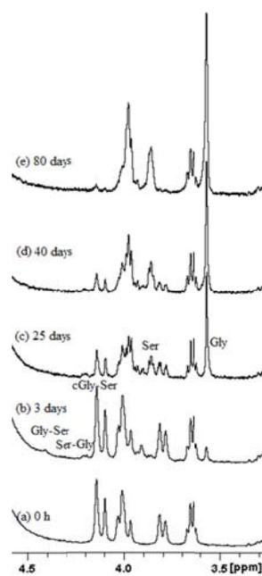
**Figure S4.**  $^1\text{H}$  NMR spectra recorded at different reaction times during the hydrolysis of 2.0 mM cGly-Ser by 2.0 mM **1** at pD 5.4 and 60 °C.
