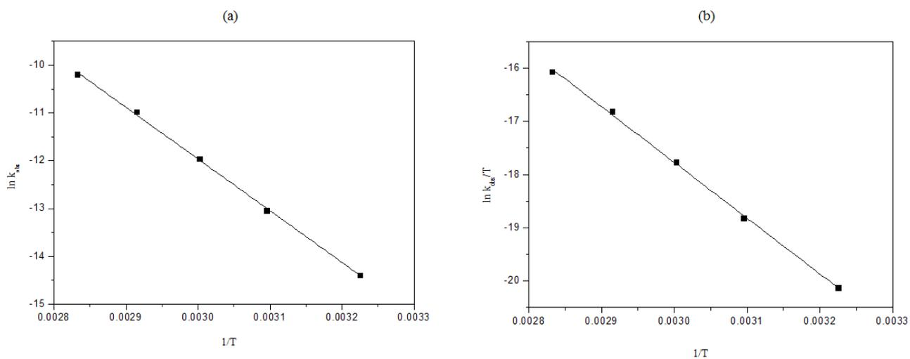
**Figure S13.** (a) Arrhenius plot of  $\ln(k_{\text{obs}})$  as a function of  $1/T$  and (b) Eyring plot of  $\ln(k_{\text{obs}}/T)$  as a function of  $1/T$  for the cleavage of 2.0 mM Gly-Ser by **1** at pH 5.4.
