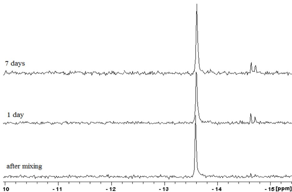
**Figure S2.**  $^{31}\text{P}$  NMR spectra of 6.0 mM **1** at 60 °C and pD 5.4, measured after mixing, after 1 day and 7 days.
