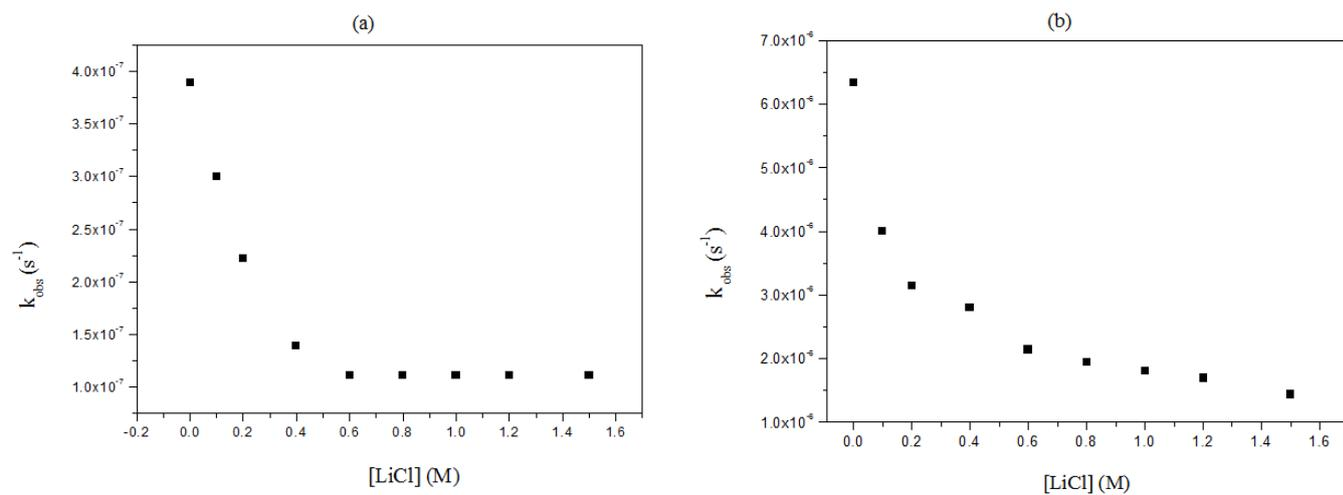
**Figure S15.** Salt effect on the rate constant of the hydrolysis of (a) 2.0 mM Gly-Gly and (b) 2.0 mM Gly-Ser in the presence of 2.0 mM **1** at pD 5.4 and 60 °C.
