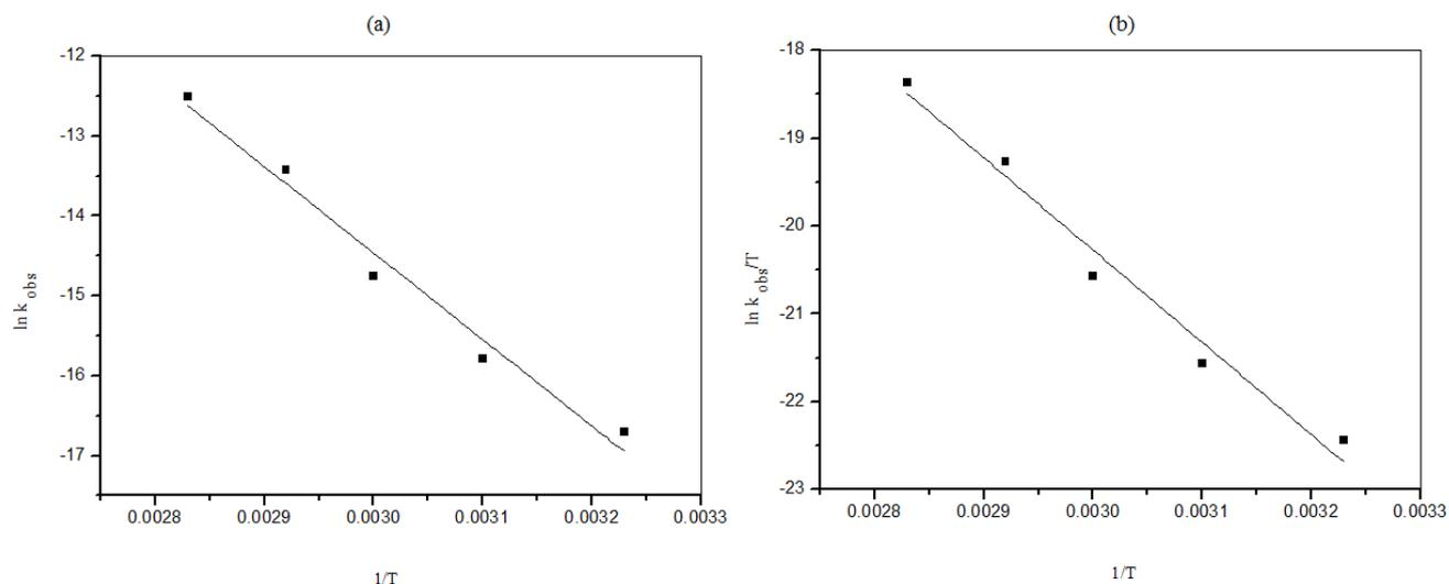
**Figure S12.** (a) Arrhenius plot of  $\ln(k_{\text{obs}})$  as a function of  $1/T$  and (b) Eyring plot of  $\ln(k_{\text{obs}}/T)$  as a function of  $1/T$  for the cleavage of 2.0 mM Gly-Gly by **1** at pH 5.4.
