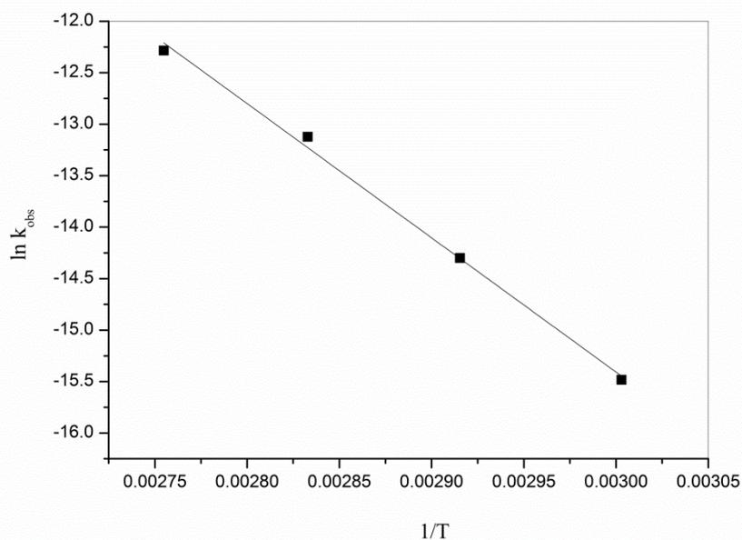
**Figure S14.** Arrhenius plot of  $\ln(k_{\text{obs}})$  as a function of  $1/T$  for the cleavage of 2.0 mM Gly-Ser in the absence of **1** at pD 5.4.
