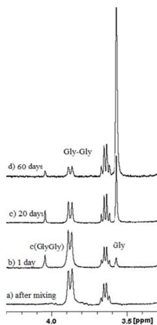
**Figure S5.** <sup>1</sup>H NMR spectra recorded at different reaction times during the hydrolysis of 2.0 mM Gly-Gly by 2.0 mM **1** at pH 5.4 and 60 °C.
