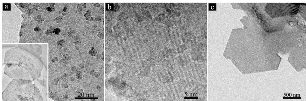
**Fig. S7** The TEM images of evolution from coarse surface to smooth nanosheets (a to c).
