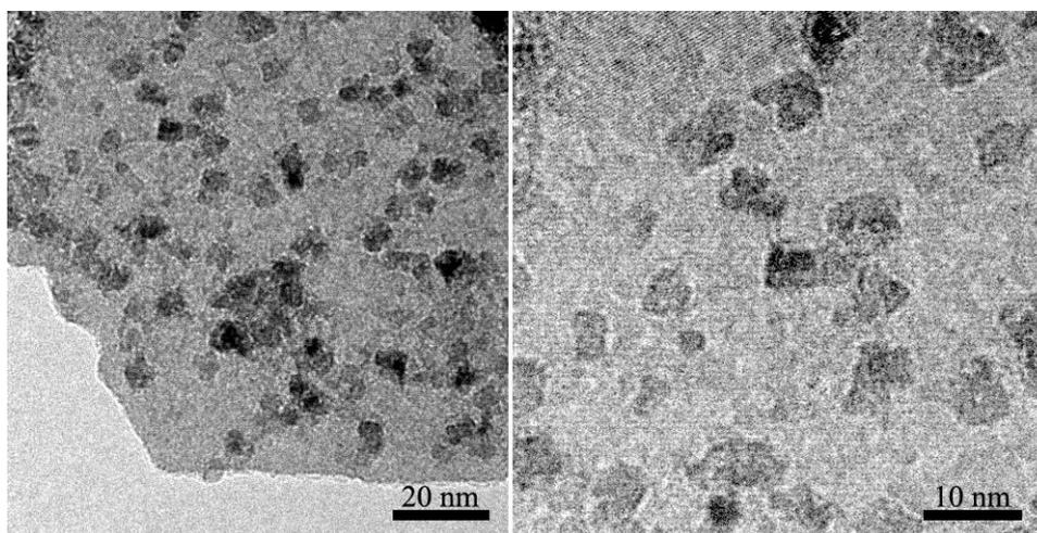
**Fig. S1** TEM images of the obtained sample after hydrothermal treatment on 1D Ce-EDA nanorods at 280 °C for 12 h.
