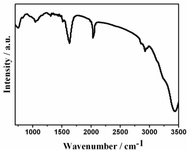
**Fig. S5** FT-IR spectrum of the sample prepared after hydrothermal treatment on 1D Ce-EDA nanorods for 6 h. The sample was collected and washed with water for 6 times.
