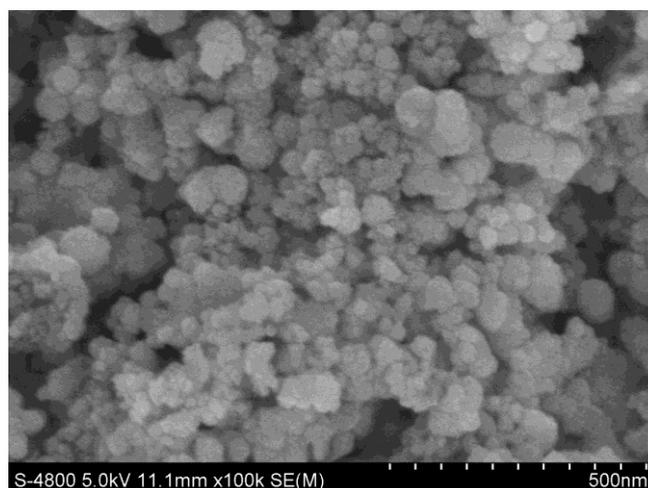
**Fig. S9** SEM image of  $\text{CeO}_2$  nanoparticles prepared by sol-gel method.
