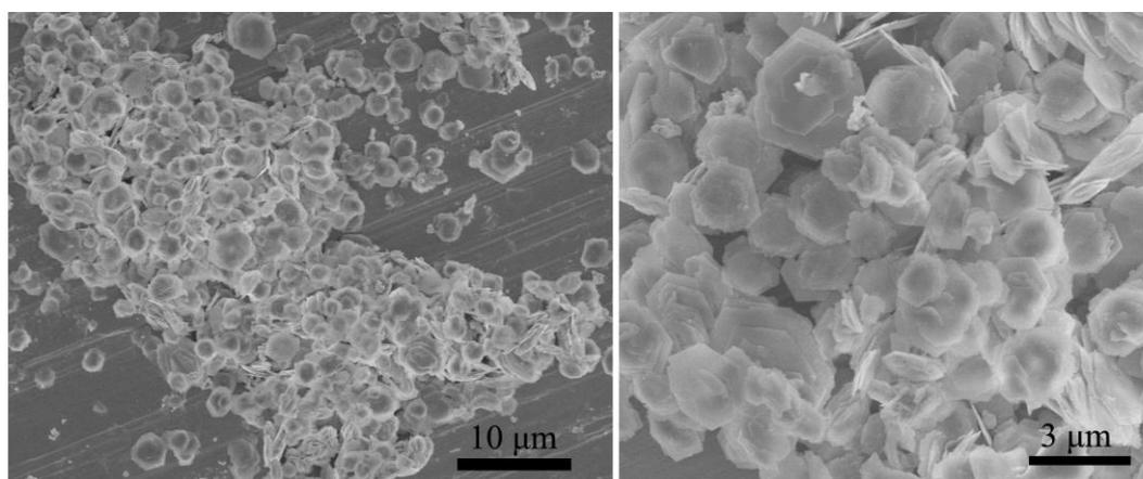
**Fig. S2** Low-magnification SEM images of the Ce(OH)CO<sub>3</sub> nanosheets.
