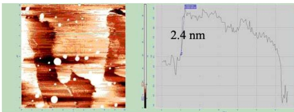
**Fig. S4** Tapping-mode AFM and corresponding photograph of the monolayer  $\text{CeO}_2$  nanosheets. Atomic force microscope (AFM) image of the  $\text{CeO}_2$  nanosheets shows that their height is  $\sim 2.4$  nm. It can be concluded that monolayer  $\text{CeO}_2$  nanosheets are derived from the thermal decomposition of single-layered  $\text{Ce}(\text{OH})\text{CO}_3$ .
