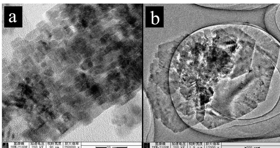
**Fig. S6** TEM images of the sample obtained in the same conditions as those for Ce(OH)CO<sub>3</sub> nanosheets except the difference in hydrothermal temperature: (a) 200 °C, (b) 240 °C.
