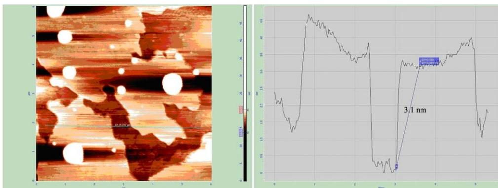
**Fig. S3** Tapping-mode AFM and corresponding photograph of the monolayer  $\text{Ce}(\text{OH})\text{CO}_3$  nanosheets on a mica plate.
