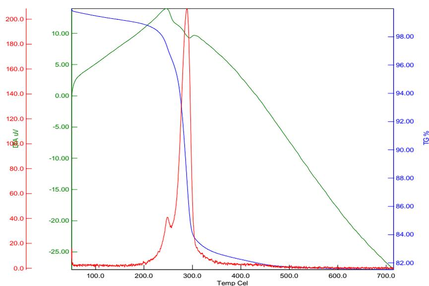
**Fig. S8** The thermogravimetric analysis curve of as-obtained  $\text{Ce}(\text{OH})\text{CO}_3$  nanosheets.
