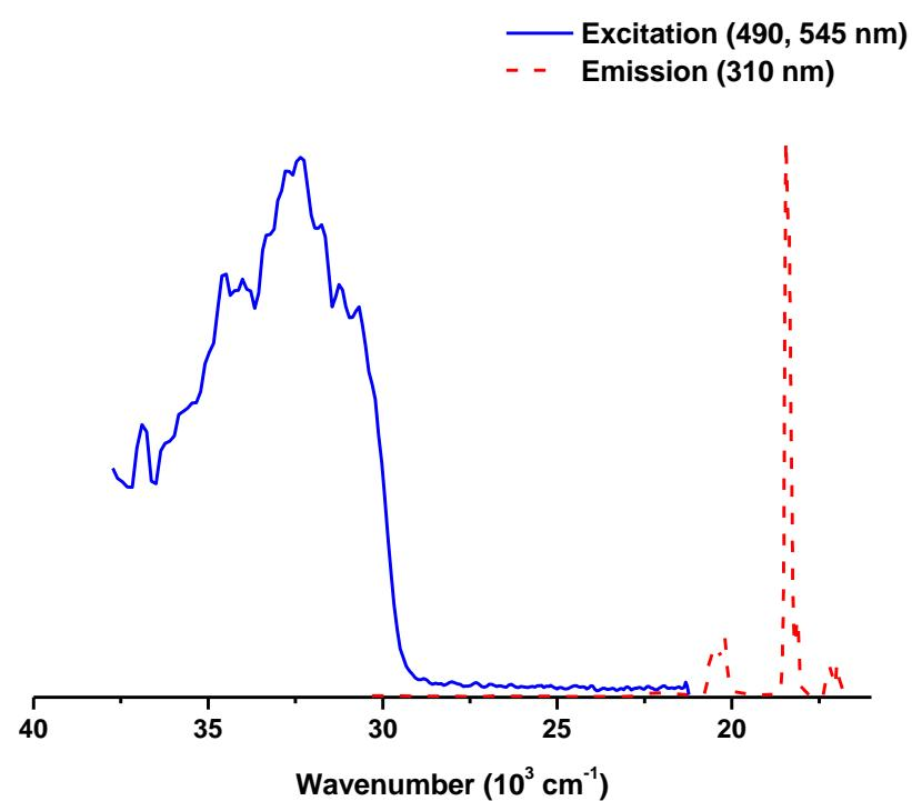
Fig. S9: Emission and excitation spectra of  $[\text{Tb}(\text{hfac})_3\text{DPEPO}]$  at 77 K in degassed DCM solution.
