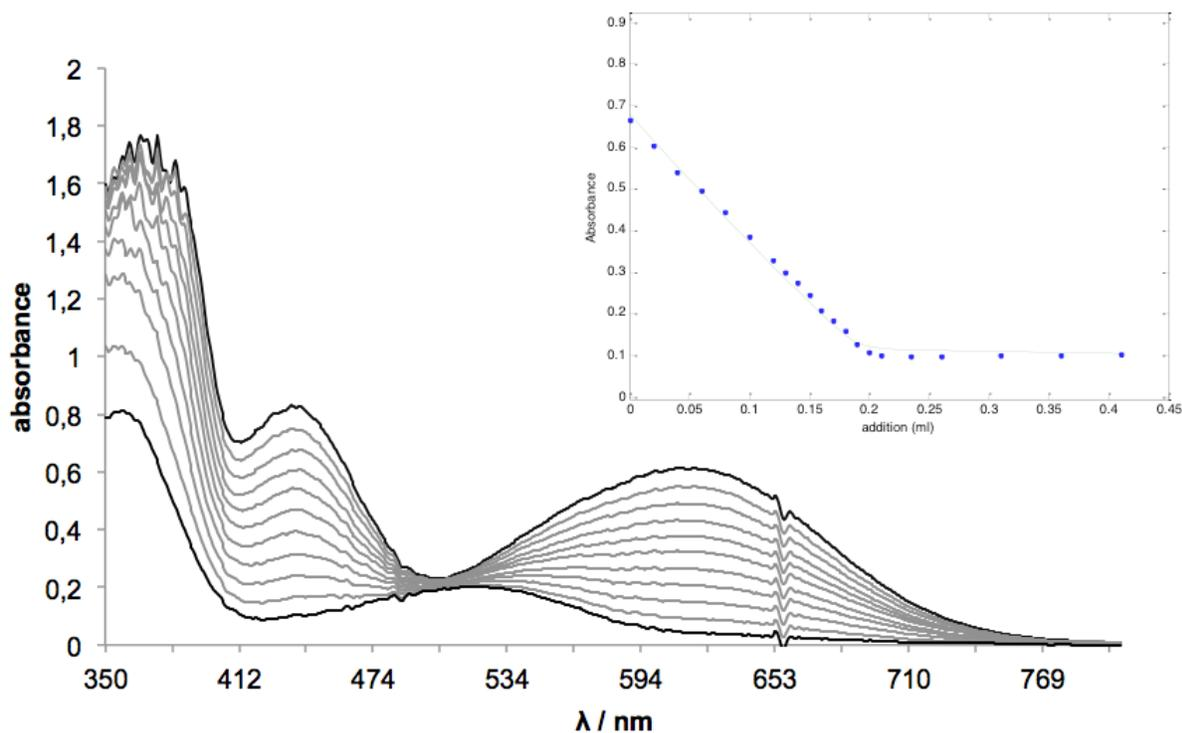
**Figure s2:** Changes in the UV-vis absorption spectrum of a solution of **2** (0.64 mM in thf) upon addition of  $[\text{Bu}_4\text{N}]\text{F} \cdot 3\text{H}_2\text{O}$ . Inset: curve fitting using ReactLab yielding  $\log K_F = 6.36(0.10)$ ,  $\sigma_r = 0.0152$ ,  $ssq = 0.291$ .
