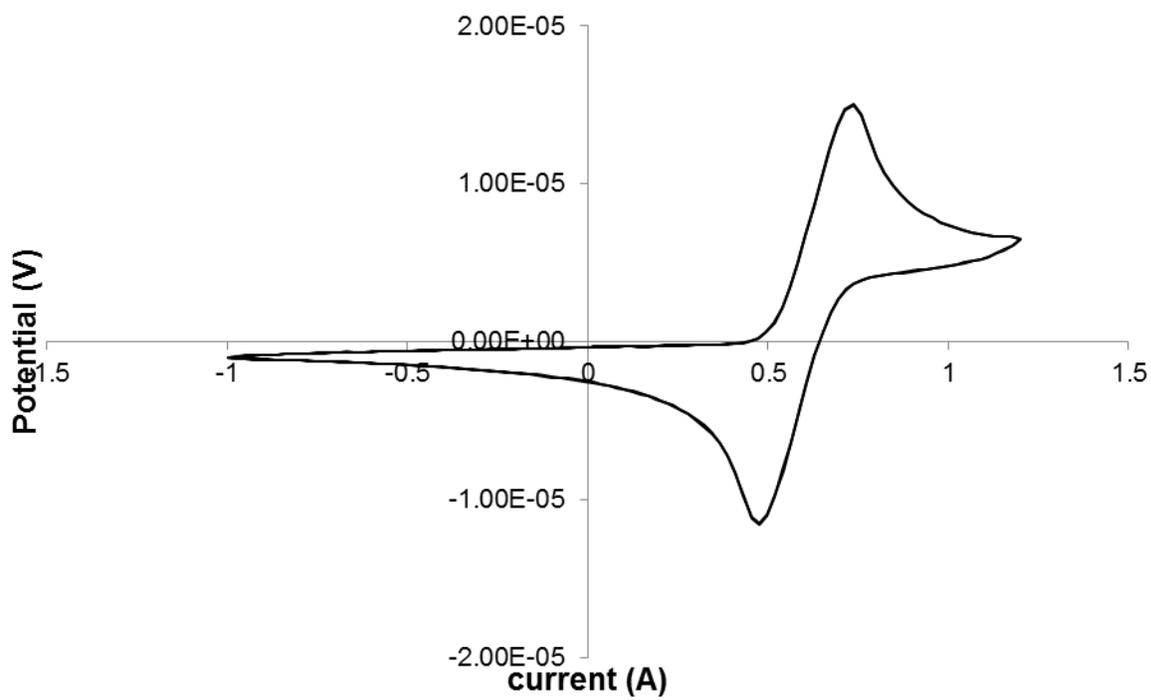
**Figure s4:** Cyclic voltammogram of **2** in thf (0.1 M  $[\text{NH}_4][\text{PF}_6]$ , scan rate:  $0.1 \text{ V s}^{-1}$ ).
