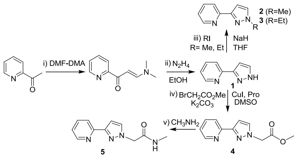
**Scheme S1.** The syntheses rout of pyrazolylpyridine-like ligands. i) DMF-DMA, 110 °C; ii) N<sub>2</sub>H<sub>4</sub>·H<sub>2</sub>O, EtOH, 85 °C; iii) RI (R=Me, Et), NaH, THF, 65 °C; iv) BrCH<sub>2</sub>CO<sub>2</sub>Me, K<sub>2</sub>CO<sub>3</sub>, Pro, DMSO, 80 °C; v) CH<sub>3</sub>NH<sub>2</sub>, RT.
