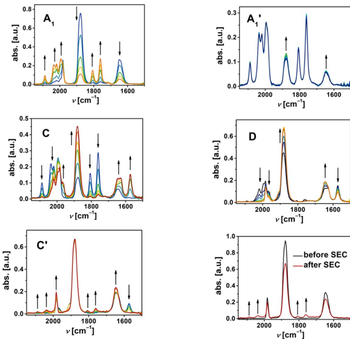
**Figure 2:** Changes in the IR spectrum of  $\text{Bu}_4\text{N}[\text{Fe}(\text{CO})_3\text{NO}]$  (**1**) in the absence of CO during various redox processes (see Scheme 2 for details). Measurements were carried out at 295 K in 0.1 M  $\text{Bu}_4\text{NPF}_6$  / THF.
