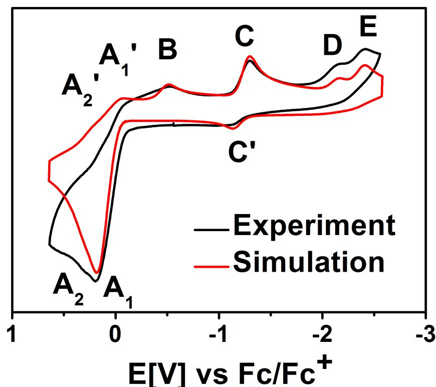
**Figure S3:** Cyclic voltammogram of  $\text{Bu}_4\text{N}[\text{Fe}(\text{CO})_3\text{NO}]$  (**1**) in THF / 0.1 M  $\text{Bu}_4\text{PF}_6$  measured at 100 mV / s at 295 K together with simulation. Ferrocene/ferrocenium was used as an internal standard.
