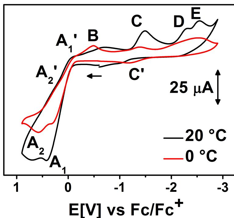
**Figure S1:** Cyclic voltammogram of  $\text{Bu}_4\text{N}[\text{Fe}(\text{CO})_3\text{NO}]$  (1) (at different temperatures) in THF / 0.1 M  $\text{Bu}_4\text{PF}_6$  measured at 100 mV/s at 295 K. Ferrocene/ferrocenium was used as an internal standard).
