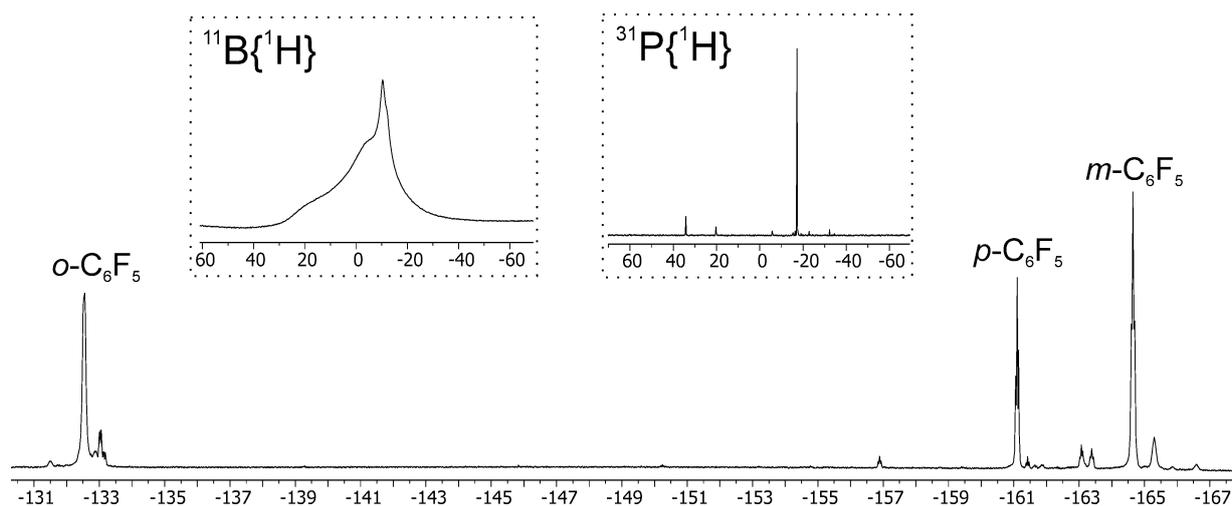
$^{19}\text{F}$  NMR (470 MHz,  $\text{C}_7\text{D}_8$ , 233 K),  $^{31}\text{P}\{^1\text{H}\}$  NMR (202 MHz,  $\text{C}_7\text{D}_8$ , 233 K) and  $^{11}\text{B}\{^1\text{H}\}$  NMR (160 MHz,  $\text{C}_7\text{D}_8$ , 233 K) of compound **3b**.
