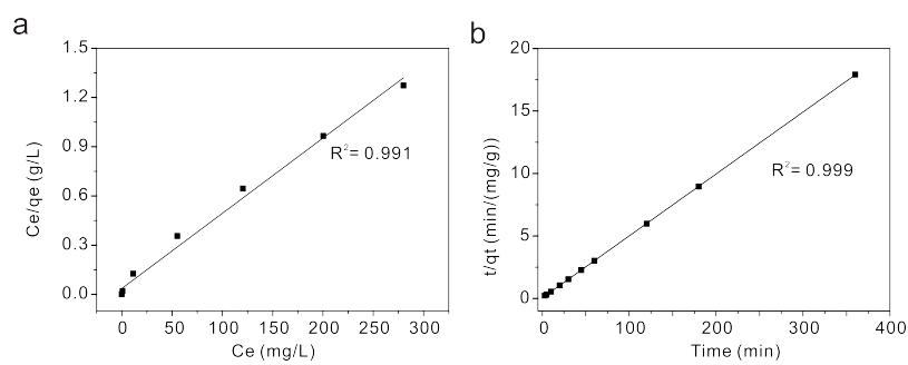
**Fig. S4** (a) Linearized Langmuir isotherms obtained from As(V) adsorption necklace-like MgO/TiO<sub>2</sub> heterojunction structures. (b) The pseudo-second-order kinetic plots for the adsorption of As(V).
