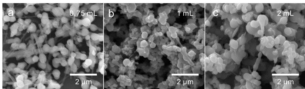
**Fig. S1** SEM images of the MgO/TiO<sub>2</sub> heterojunction structures prepared using 0.75 mL(a), 1 mL (b), and 2 mL (c) of TBT.
