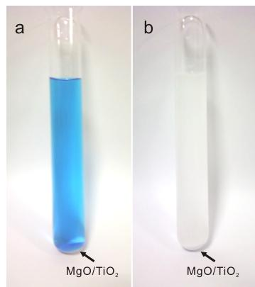
**Fig. S5** The digital photographs of the MgO/TiO<sub>2</sub> heterojunction structures dispersed in MB solution before (a) and after (b) UV irradiation.
