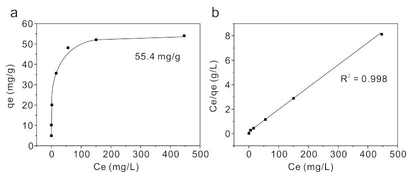
**Fig. S6** Adsorption isotherm (a) and linearized Langmuir isotherm (b) obtained from As(V) adsorption onto MgO/TiO<sub>2</sub> heterojunction structures after degradation of MB dye under UV irradiation.
