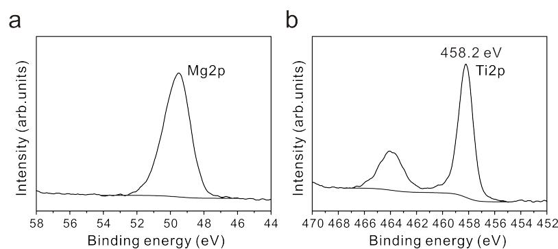
**Fig. S3** XPS Mg<sub>2p</sub> and Ti<sub>2p</sub> spectra of the MgO/TiO<sub>2</sub> heterojunction structures.
