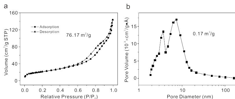
**Fig. S2** Nitrogen adsorption–desorption isotherm (a) and the BJH–PSD pore size distributions (b) of the necklace-like MgO/TiO<sub>2</sub> heterojunction structures.
