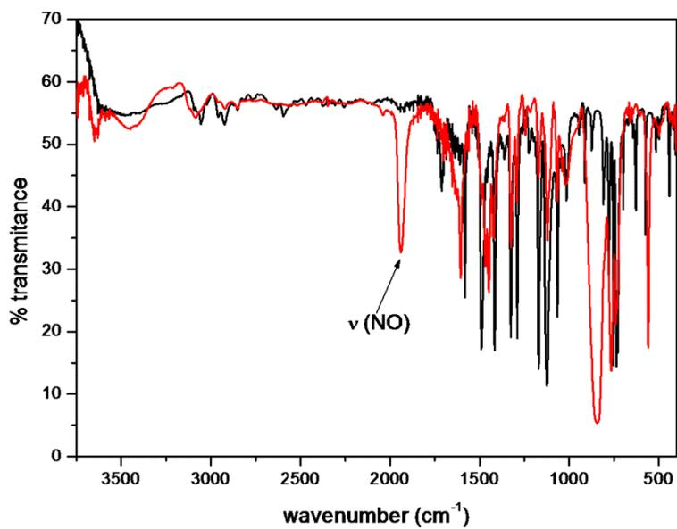
Figure 1: FTIR spectrum of  $[\text{Ru}(\text{pc})(\text{pz})_2]$  (black line) and  $[\text{Ru}(\text{pc})(\text{pz})_2\{\text{Ru}(\text{bpy})_2(\text{NO})\}_2](\text{PF}_6)_6$  (red line) in KBr pellet.
