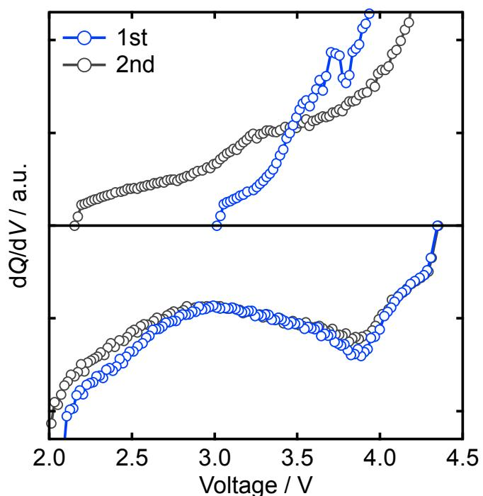
Figure S3 Incremental capacity  $dQ/dV$  versus the cell voltage. Upper and lower show the charging and the discharging process respectively.
