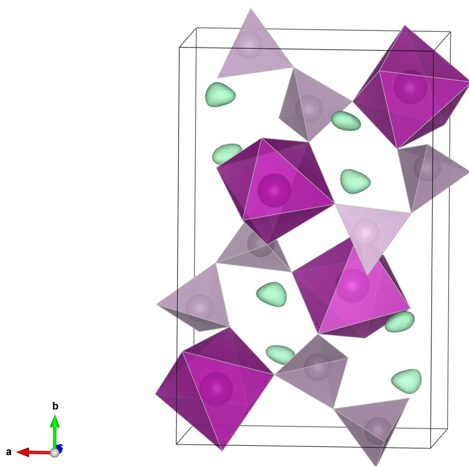
Figure S2 Isosurface of difference Fourier synthesis map drown with  $[\text{MnP}_2\text{O}_7]^{2-}$  framework structure. The isosurface value is  $0.7 \text{ \AA}^{-3}$ . The map was calculated without lithium to determine the lithium positions. This figure is drown with a computer program VESTA (K. Momma et al., *J. Appl. Cryst.*, 41(3): 653–658)
