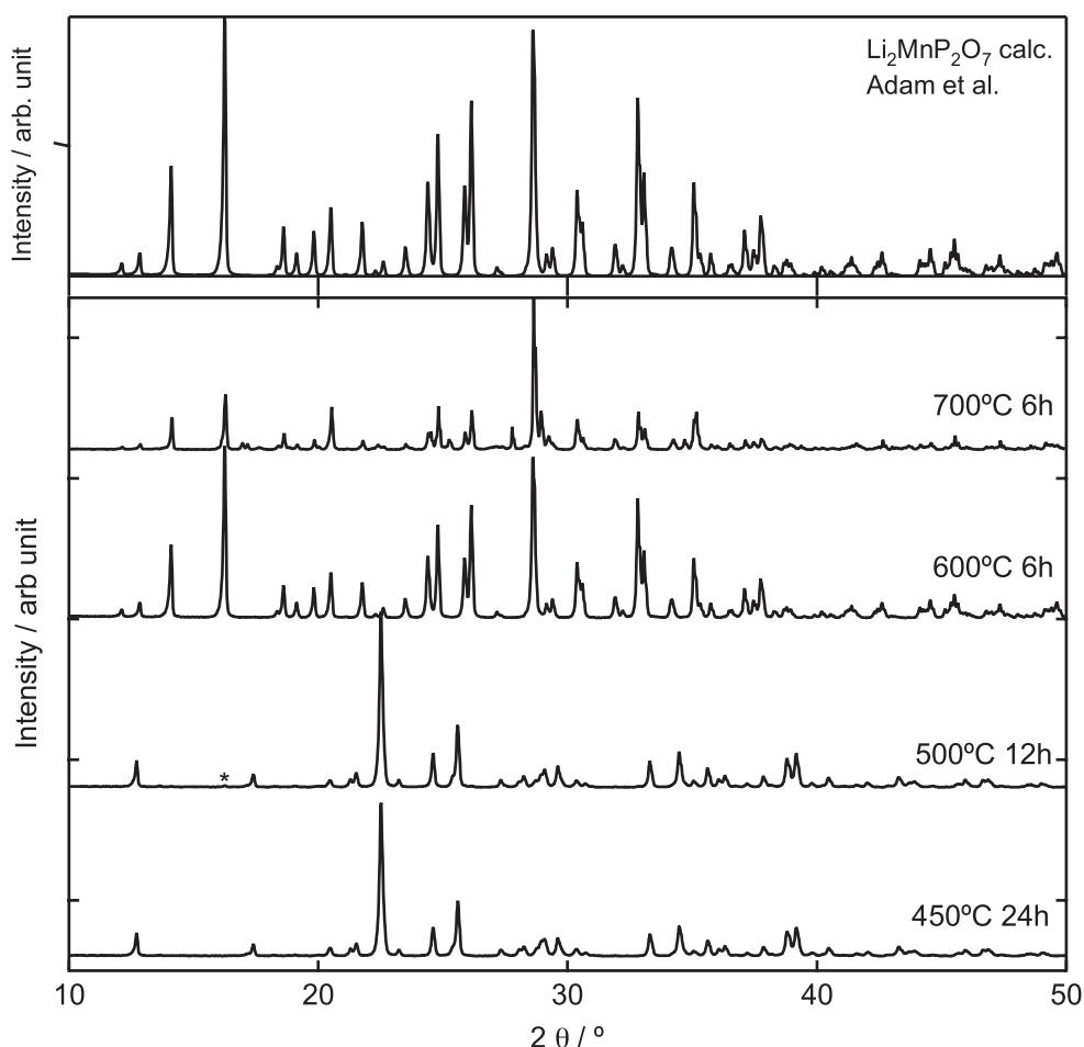
Figure S1 Powder X-ray diffraction patterns of the  $\text{Li}_2\text{MnP}_2\text{O}_7$  samples.
