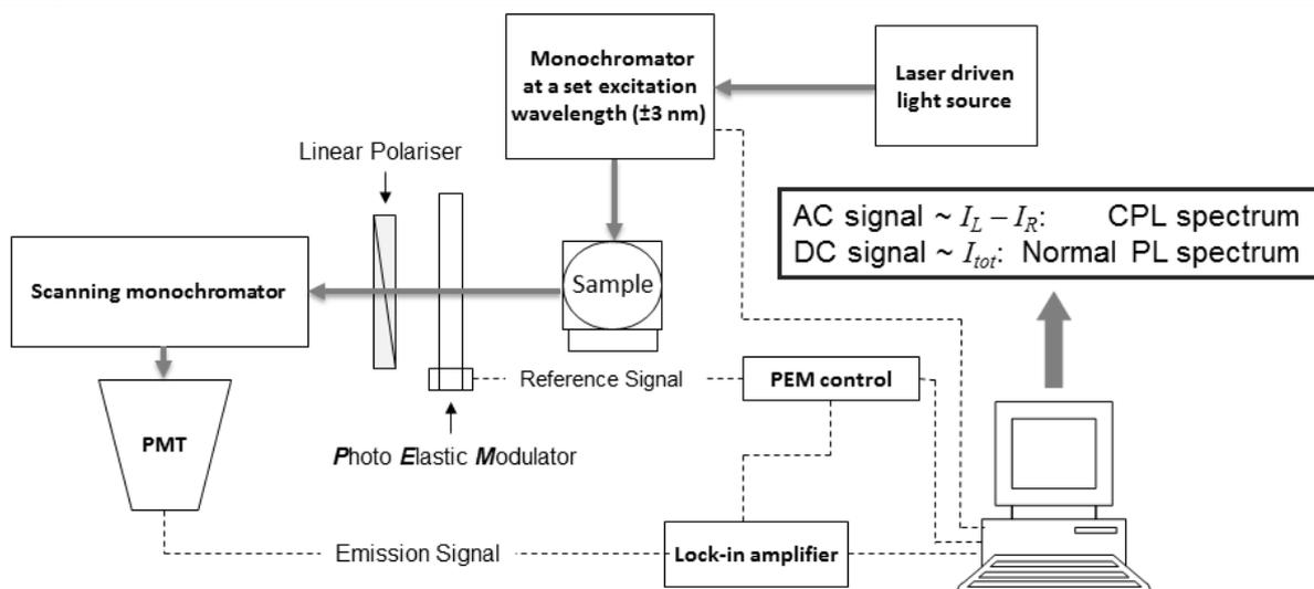
Figure S1: Schematic diagram of CPL instrumentation.
