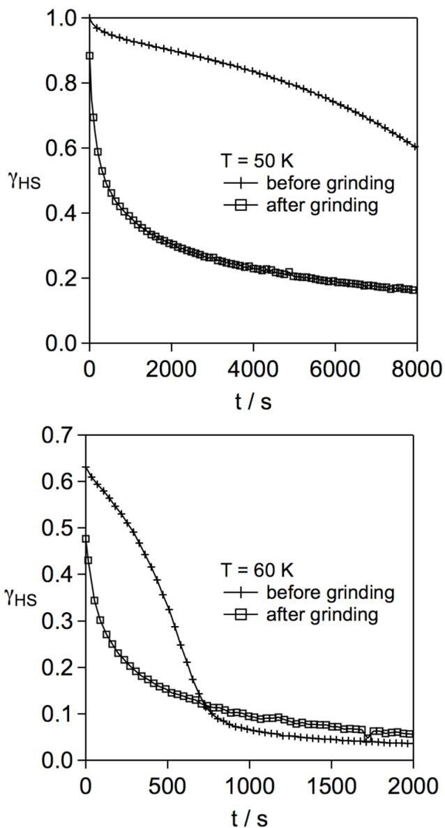
**Figure S5.** HS-LS relaxation curves registered on  $[\text{Fe}(\text{mepy})_3\text{tren}](\text{PF}_6)_2 \cdot \text{C}_7\text{H}_8 \cdot \text{C}_2\text{H}_3\text{N}$  crystals at 50 and 60 K before (+) and after ( $\square$ ) grinding.
