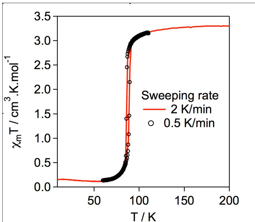
**Figure S3.** Evolution of the product of the magnetic susceptibility by the temperature  $\chi_M T$  vs. temperature  $T$  registered at 2 K/min between 10 and 200 K and at 0.5 K/min between 60 and 110 K on  $[\text{Fe}(\text{mepy})_3\text{tren}](\text{PF}_6)_2 \cdot \text{C}_7\text{H}_8 \cdot \text{C}_2\text{H}_3\text{N}$  single crystals.
