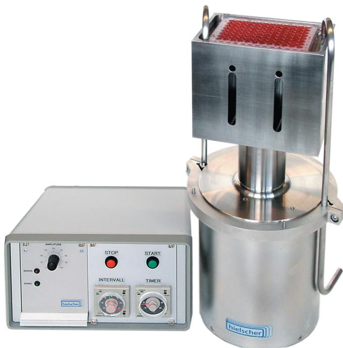
**Fig. S11** Utilised HT ultrasonic device UIO250MTP by Hielscher. Picture provided by the company.
