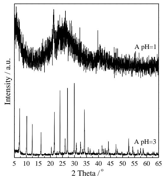
**Figure S1** X-ray diffraction pattern: zeolite A was immersed in distilled water with different pH.
