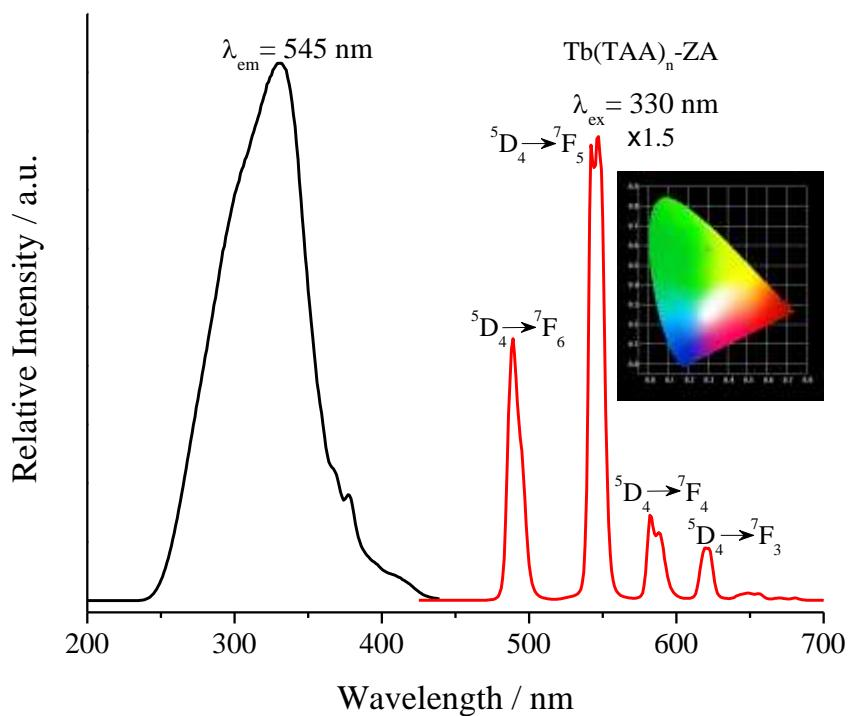
**Figure S7** The excitation (black line) and emission spectra (red line) of  $\text{Tb}(\text{TAA})_n\text{-ZA}$ . The point of emission spectra in CIE chromaticity diagram is in the area of green (CIE x: 0.3032; CIE y: 0.5823).
