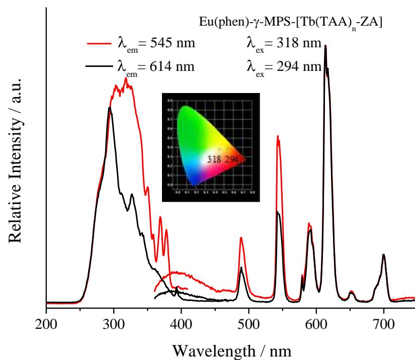
**Figure S10** The excitation (black line 614 nm and red line 545 nm) and emission spectra (black line 294 nm and red line 318 nm) of Eu(phen)- $\gamma$ -MPS-[Tb(TAA)<sub>n</sub>-ZA].
