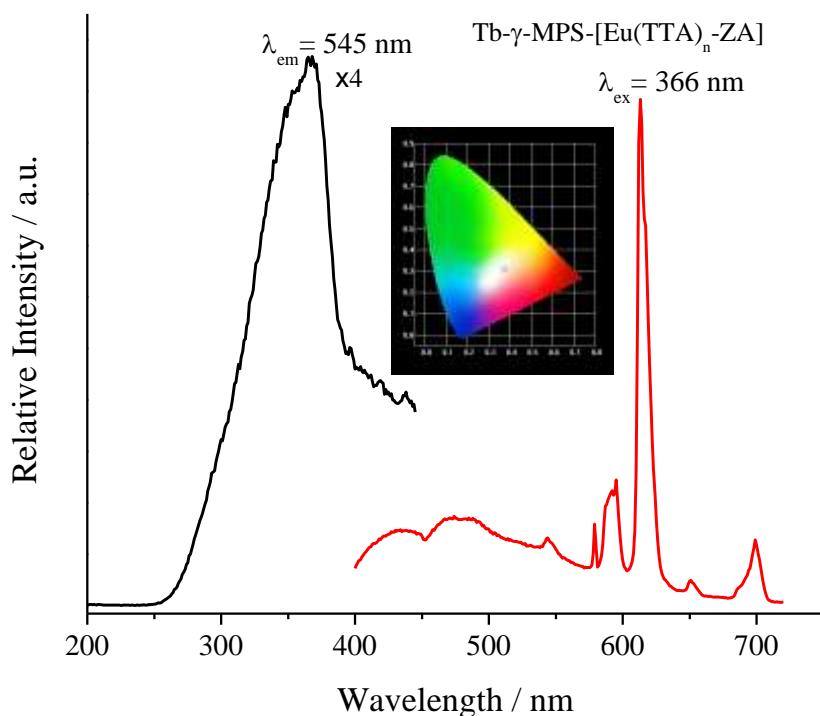
**Figure S8** The excitation (black line) and emission spectra (red line) of  $\text{Tb}-\gamma\text{-MPS-}[\text{Eu}(\text{TTA})_n\text{-ZA}]$ . Before introducing phen or bipy ligands, the band at 550 nm which is the emission of  $\text{Tb}^{3+}$  is rather weak. And the point of emission spectra in CIE chromaticity diagram is in the area of white (CIE x: 0.3727; CIE y: 0.3094).
