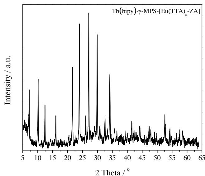
**Figure S2** X-ray diffraction pattern of the final hybrid material of  $\text{Tb}(\text{bipy})\text{-}\gamma\text{-MPS-[Eu(TTA)}_n\text{-ZA]}$ .
