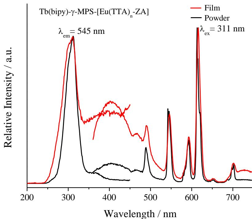
**Figure S14** The excitation and emission spectra of  $\text{Tb}(\text{bipy})\text{-}\gamma\text{-MPS-[Eu(TTA)}_n\text{-ZA}]$  (red line: film, black line : powder).
