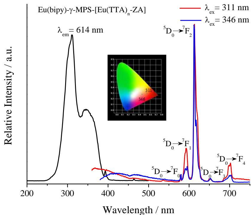
**Figure S11** The excitation (black line) and emission spectra (red line 311 nm and blue line 346 nm) of Eu(bipy)- $\gamma$ -MPS-[Eu(TTA)<sub>n</sub>-ZA].
