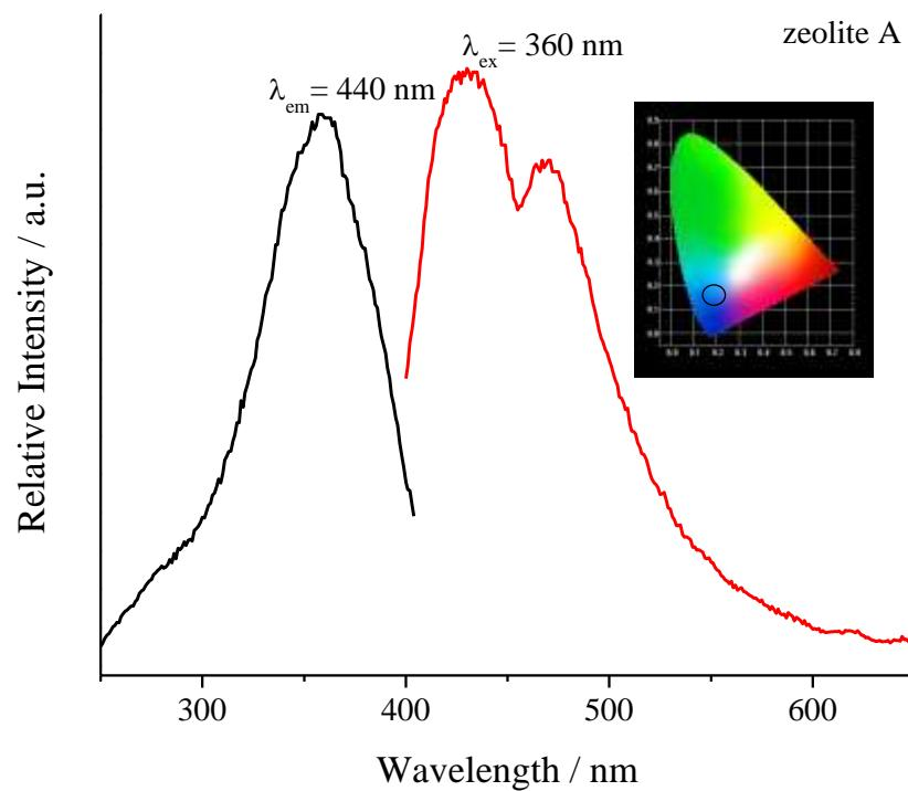
**Figure S3** The excitation (black line) and emission spectra (red line) of zeolite A. The point of emission spectra in CIE chromaticity diagram is in the area of blue (CIE x: 0.1748; CIE y: 0.1597).
