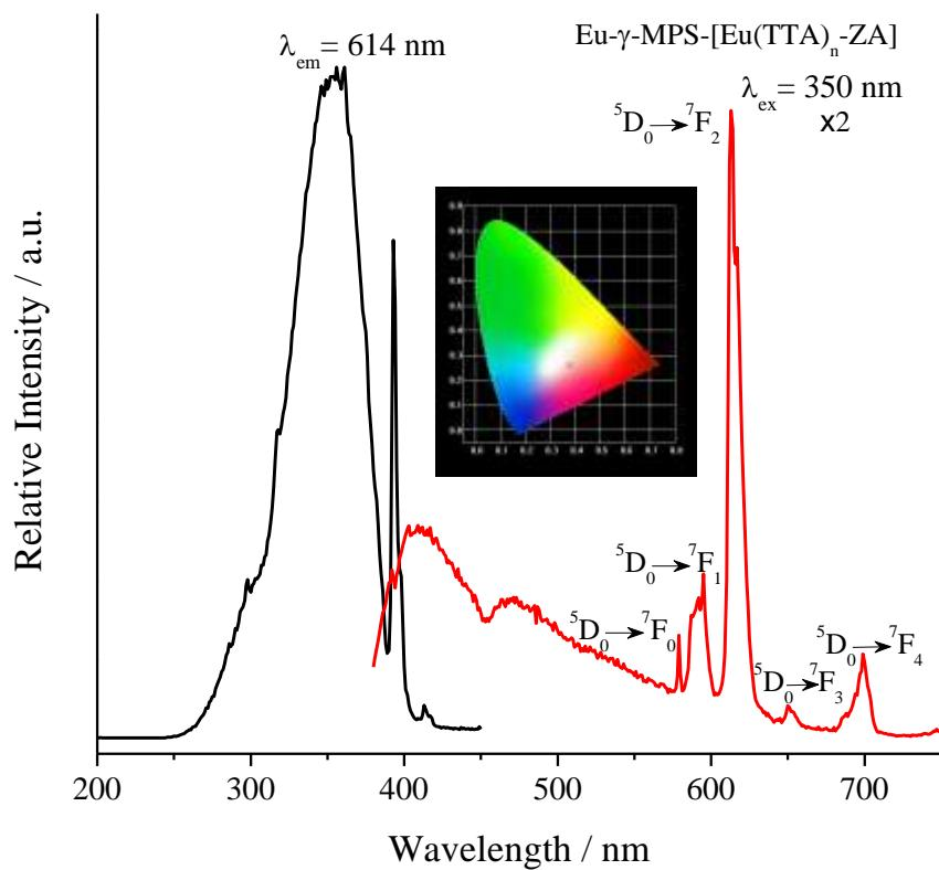
**Figure S9** The excitation (black line) and emission spectra (red line) of Eu- $\gamma$ -MPS-[Eu(TTA)<sub>n</sub>-ZA]. The point of emission spectra in CIE chromaticity diagram is in the area of green (CIE x: 0.3333; CIE y: 0.2633).
