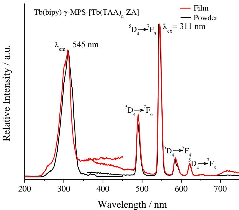
**Figure S16** The excitation and emission spectra of Tb(bipy)- $\gamma$ -MPS-[Tb(TAA)<sub>n</sub>-ZA] (red line: film, black line : powder).
