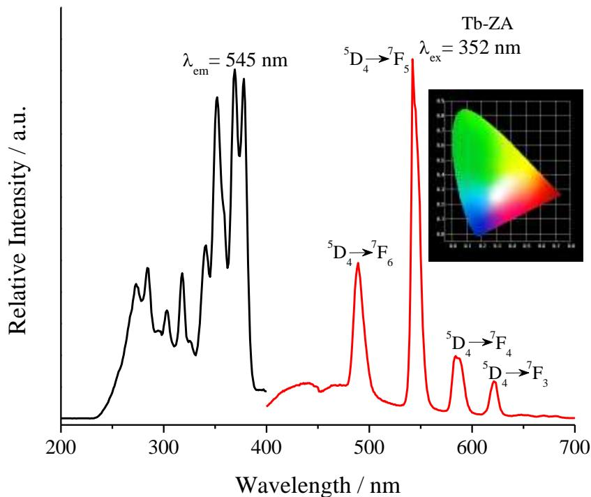
**Figure S6** The excitation (black line) and emission spectra (red line) of Tb-ZA. The point of emission spectra in CIE chromaticity diagram is in the area of green (CIE x: 0.2605; CIE y: 0.4217).
