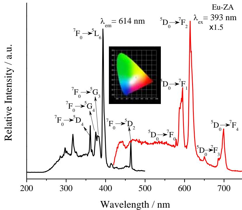
**Figure S4** The excitation (black line) and emission spectra (red line) of Eu-ZA. The point of emission spectra in CIE chromaticity diagram is in the area of white (CIE x: 0.3872; CIE y: 0.3489).
