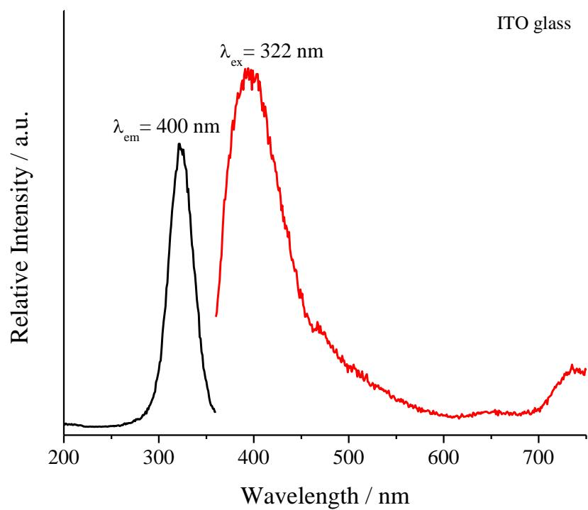
**Figure S13** The excitation (black line) and emission spectra (red line) of pure ITO glass which is the substrate of the film.
