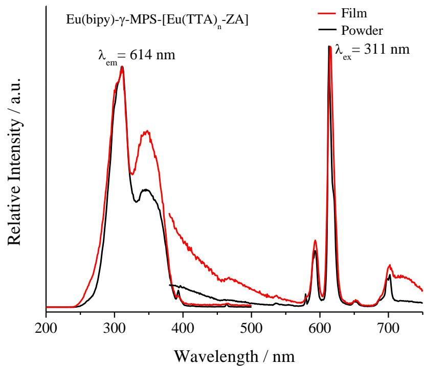
**Figure S15** The excitation and emission spectra of Eu(bipy)- $\gamma$ -MPS-[Eu(TTA)<sub>n</sub>-ZA] (red line: film, black line : powder).
