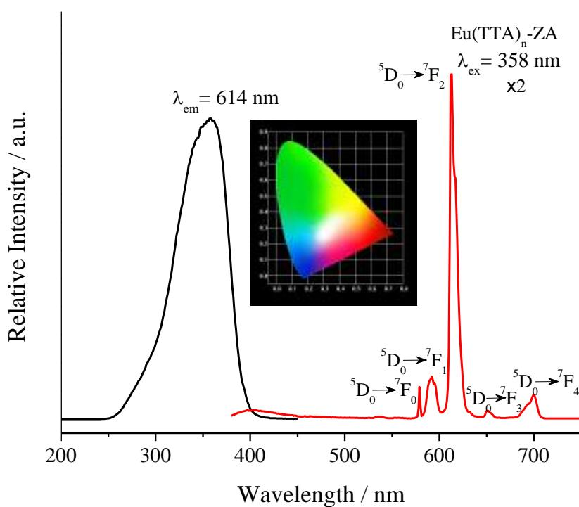
**Figure S5** The excitation (black line) and emission spectra (red line) of Eu(TTA)<sub>n</sub>-ZA. The point of emission spectra in CIE chromaticity diagram is in the area of red (CIE x: 0.6114; CIE y: 0.3213).
