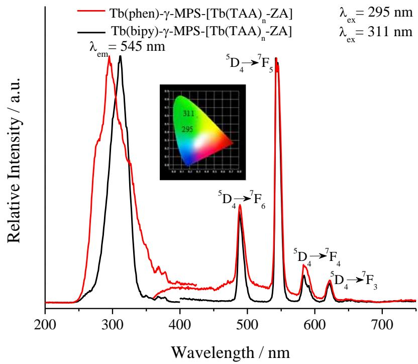
**Figure S12** The excitation and emission spectra of Tb(phen)- $\gamma$ -MPS-[Tb(TAA)<sub>n</sub>-ZA] (red line) and Tb(bipy)- $\gamma$ -MPS-[Tb(TAA)<sub>n</sub>-ZA] (black line).
