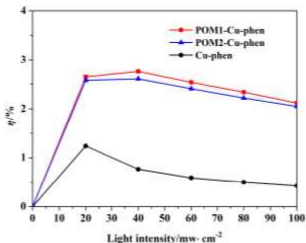
**Fig. S2** Relationship between light intensity and energy conversion efficiencies of DSSCs containing POM1-Cu-phen, POM2-Cu-phen and Cu-phen as the redox couples.
