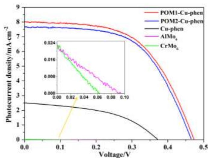
**Fig. S1** Photocurrent density-Voltage curves of DSSCs with POM1-Cu-phen, POM2-Cu-phen, Cu-phen redox couples and AlMo<sub>6</sub>-only, CrMo<sub>6</sub>-only based electrolytes. The insert shows the amplification of axis.
