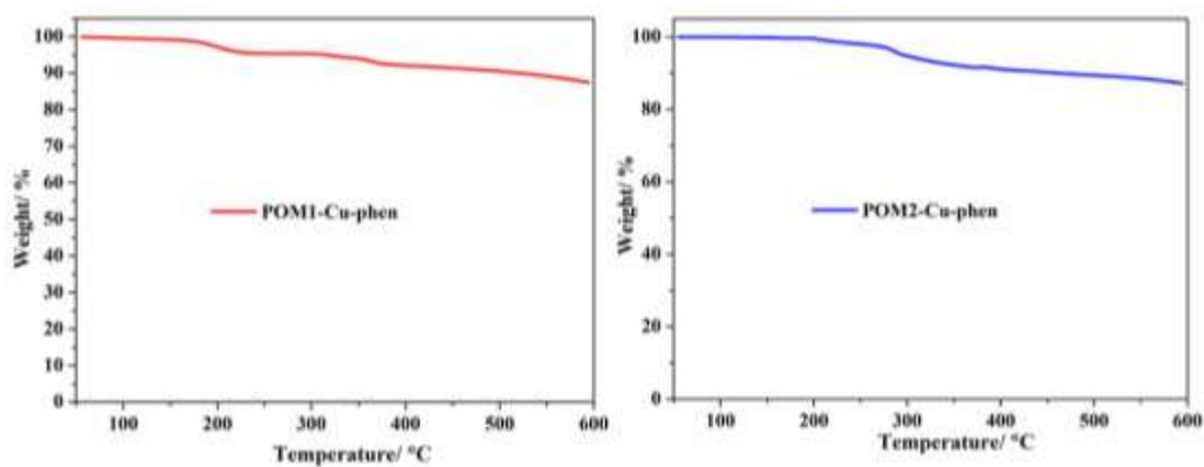
**Fig. S5** The TG curve of POM1/POM2-Cu-phen.
