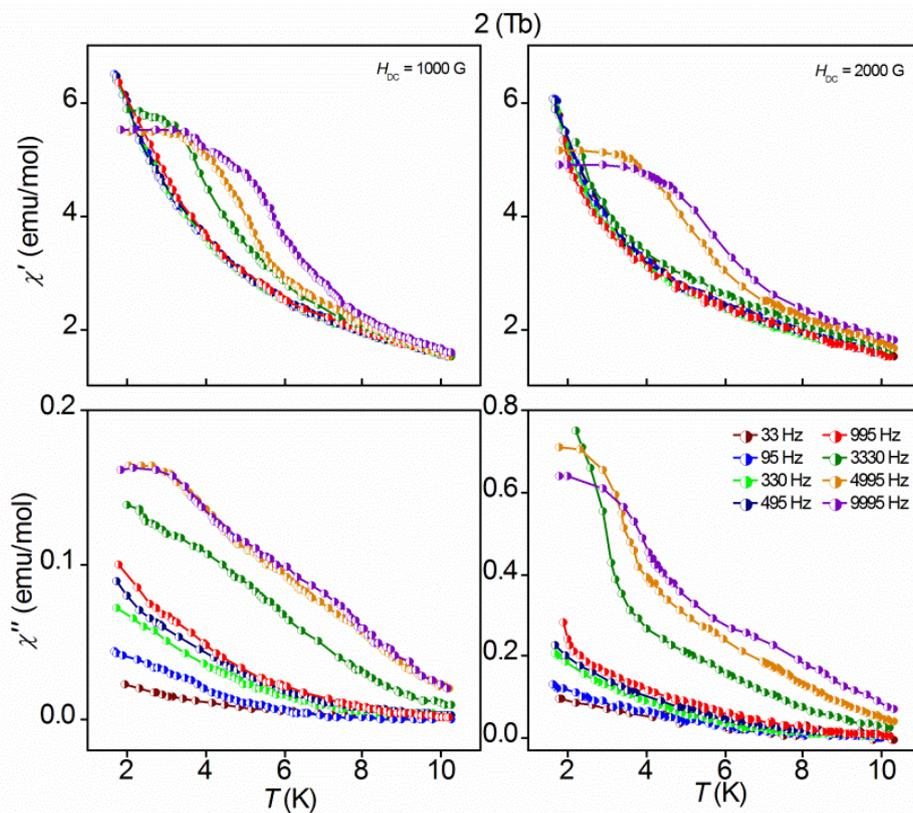
**Fig. S5** Temperature dependence of the in-phase,  $\chi'$ , and out-of-phase,  $\chi''$ , components of the AC magnetic susceptibility of **2** under applied static fields of 1 and 2 kG at different frequencies.
