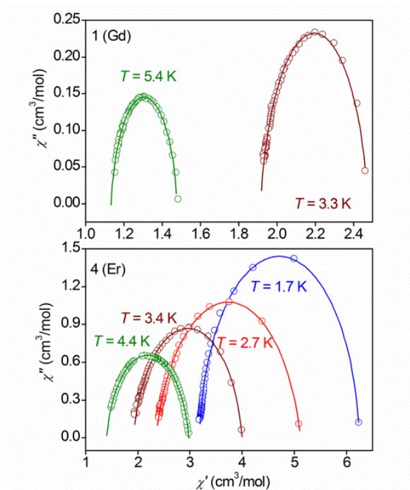
**Fig. S7** Cole–Cole plots of  $\chi''$  vs.  $\chi'$  of **1** (top) and **4** (bottom). The solid lines represent a least-squares fitting of the data to a distribution of single relaxation processes (Eq. 1).
