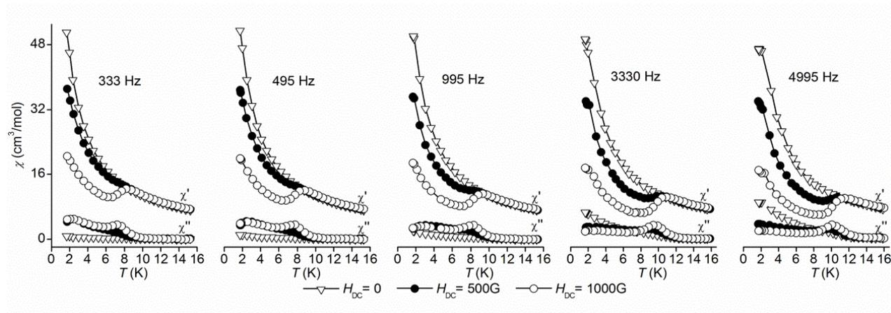
**Fig. S6** Plots of the in-phase,  $\chi'$ , and out-of-phase,  $\chi''$ , AC susceptibility for compound **3** as a function of temperature at fixed frequencies 333, 495, 995, 3330 and 4995 Hz (AC field with amplitude of 10 Oe and static fields  $H_{DC}$  of 0 G, 500 G and 1000 G).
