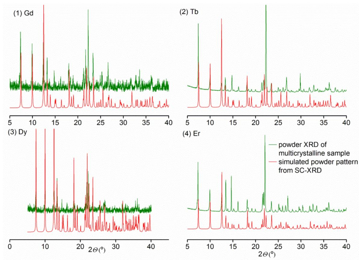
**Fig. S1** Powder X-ray diffraction patterns for compounds **1**, **2**, **3** and **4**. Comparison between simulated powder patterns from the SC-XRD structure and powder XRD data.
