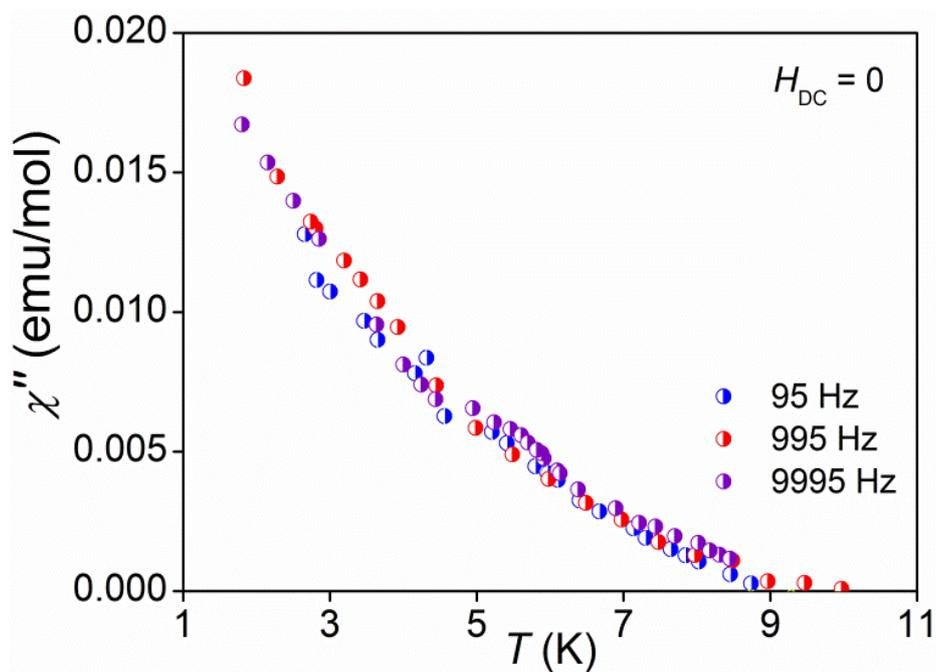
**Fig. S4** Temperature dependence of the out-of-phase component of the AC magnetic susceptibility,  $\chi''$ , of **1** without an applied static field, at different frequencies.
