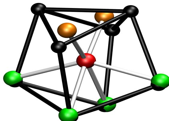
**Figure S3a:** Superimposition of a dodecahedron (black) and the metal fragment  $[\text{PtZn}_4\text{P}_2]$  extracted from the molecular structure of **3b** (coloured), concerning Zn atoms
