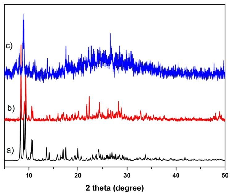
**Fig. S14** The simulated (a) and experimental powder X-ray diffraction patterns for the fresh (b) and the used (c) catalyst **2**
