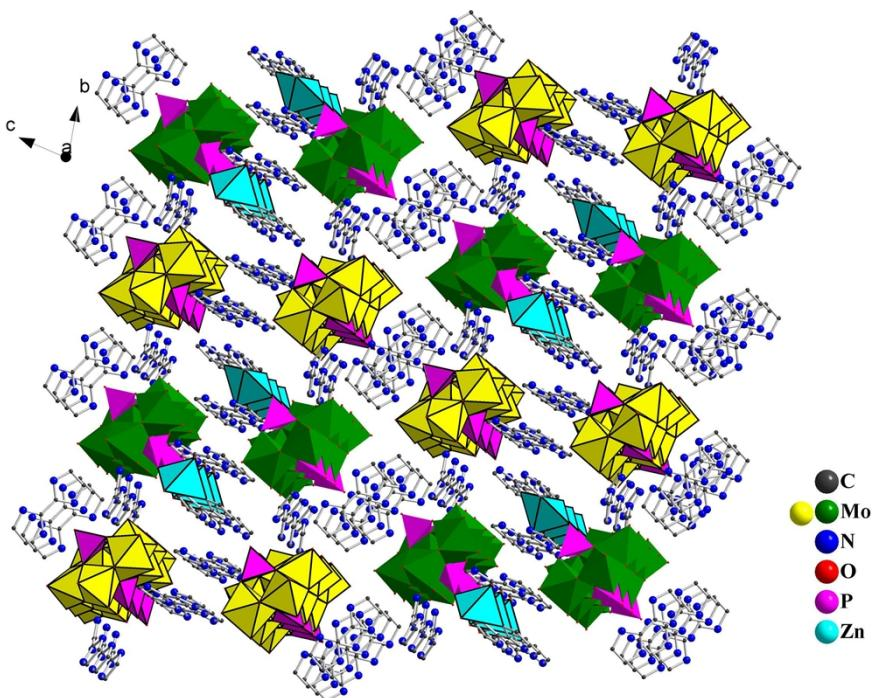
**Fig. S6** The packing view of **3** (The green part: Zn- $\{\text{P}_2\text{Mo}_5\}$ ; the yellow part:  $\{\text{P}_2\text{Mo}_5\}$ , free  $\text{H}_2\text{O}$  molecules, and hydrogen atoms have been omitted for clarity)
