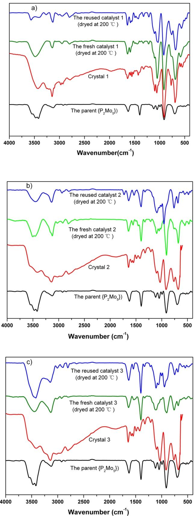
**Fig. S13** Comparisons of IR spectra of the parent  $\{\text{P}_2\text{Mo}_5\}$ , the crystal, and the fresh and the used catalysts 1/2/3 (a/b/c).
