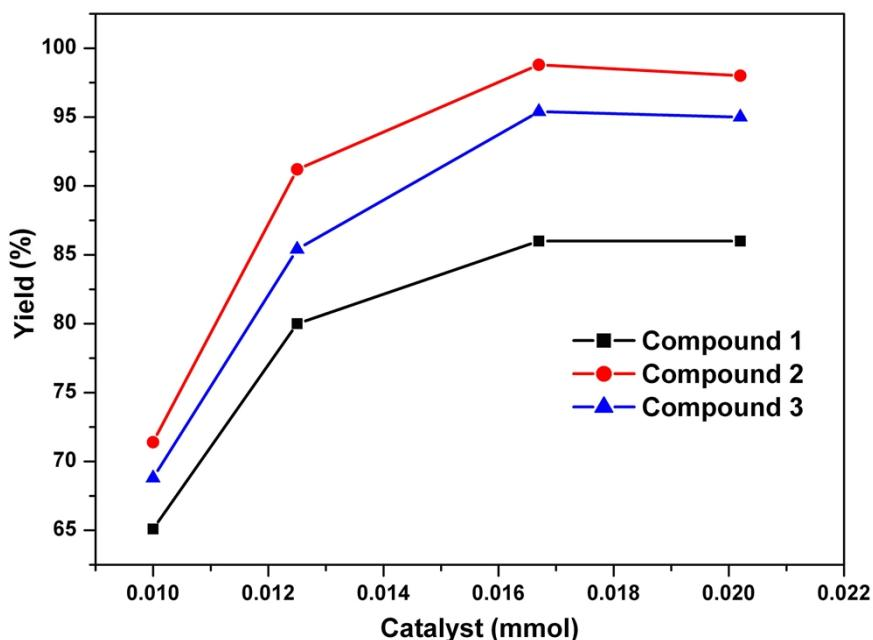
**Fig. S11** Effect of the amount of **1/2/3** on cyclohexanone ethylene ketal yield: cyclohexanone/glycol molar ratio, 1:1.4; reaction temperature, 95–100 °C; reaction time, 2 h; water-carrying agent, cyclohexane (10 mL).
