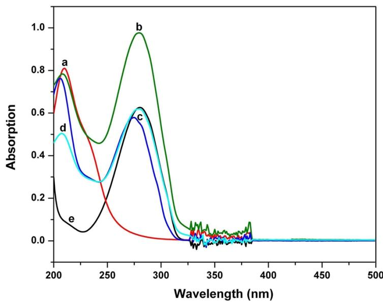
**Fig. S1** Comparison of UV-visible spectra for the parent  $\{P_2Mo_5\}$ ,  $ZnSO_4$ ,  $H_2biim$  and **1-3** ( $5 \times 10^{-5} \text{ mol L}^{-1}$ ) at pH = 6-7 aqueous solutions. In the synthetic process of **1-3**, the pH controlling is very important. When the crystal products **1-3** redissolved in aqueous solution (pH = 6-7), the skeleton of  $\{P_2Mo_5\}$  may be transformed to that of  $\{P_4Mo_6\}$  according the UV spectra analysis and the literatures<sup>1-3</sup>
