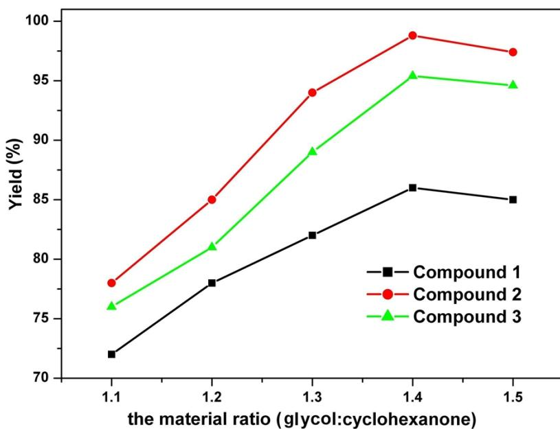
**Fig. S10** Effect of the material ratio on cyclohexanone ethylene ketal yield: catalyst (of Mo)/cyclohexanone molar ratio, 1:300; reaction temperature, 95-100 °C; reaction time, 2 h. water-carring agent, cyclohexane (10 mL)
