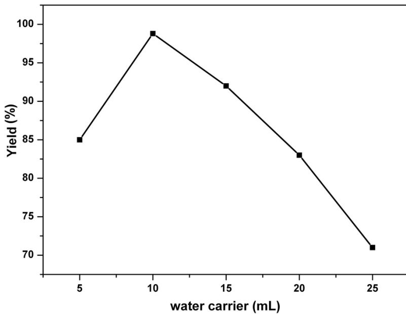
**Fig. S12** Effect of the amount of water-carrying agent on cyclohexanone ethylene ketal yield: cyclohexanone/glycol molar ratio, 1:1.4; catalyst (compound **2**, of Mo)/cyclohexanone molar ratio, 1:300; reaction time, 2 h
