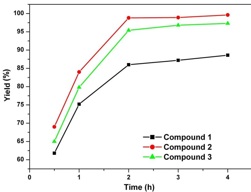
**Fig. S9** Effect of reaction time on cyclohexanone ethylene ketal yield: cyclohexanone/glycol molar ratio, 1:1.4; catalyst (of Mo)/cyclohexanone molar ratio, 1:300; reaction temperature, 95-100 °C; water-carring agent, cyclohexane (10 mL)
