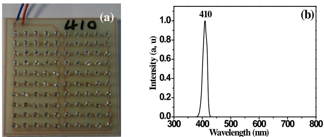
**Fig.S1** (a) photograph of LED arrays and (b) the wavelength spectrum of LED lamp
