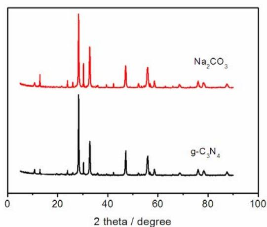
Fig. S3 XRD patterns of the Bi<sub>2</sub>O<sub>2</sub>CO<sub>3</sub>/Bi<sub>2</sub>WO<sub>6</sub> nanocomposites prepared using g-C<sub>3</sub>N<sub>4</sub> or Na<sub>2</sub>CO<sub>3</sub> as a source of CO<sub>3</sub><sup>2-</sup>.
