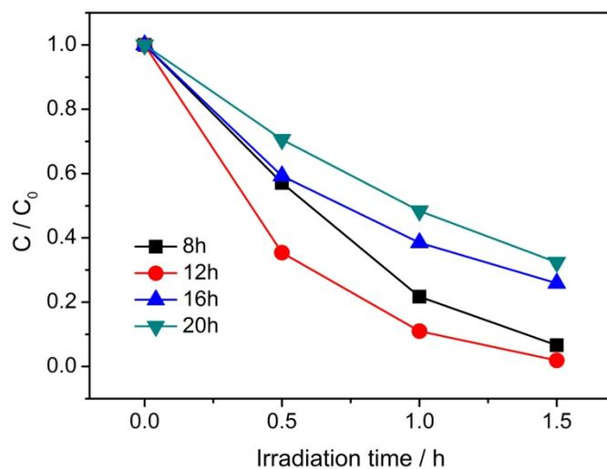
Fig. S11 Comparison of photocatalytic activity of the  $\text{Bi}_2\text{O}_2\text{CO}_3/\text{Bi}_2\text{WO}_6$  composites attained after reaction for (A) 8 h, (B) 12 h, (C) 16 h, and (D) 20 h towards the degradation of RhB under visible light irradiation.
