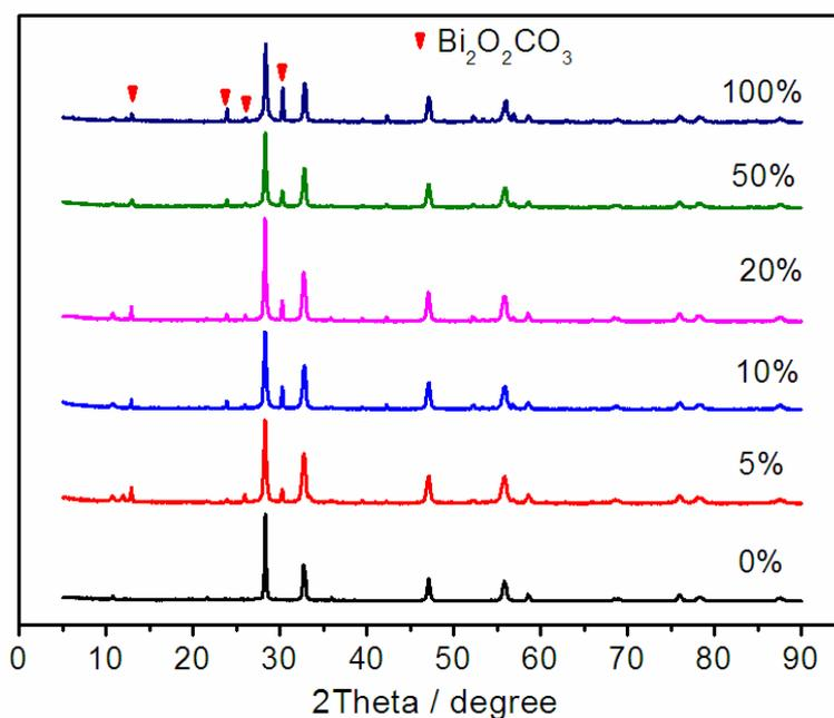
Fig. S6 XRD patterns of the  $\text{Bi}_2\text{O}_2\text{CO}_3/\text{Bi}_2\text{WO}_6$  composites prepared using different amounts of  $\text{g-C}_3\text{N}_4$ .
