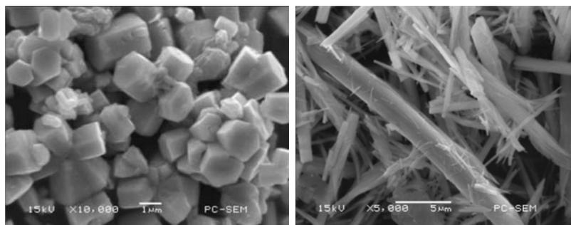
Fig. S2 SEM images of the ZnO samples obtained with g-C<sub>3</sub>N<sub>4</sub> as a source of NH<sub>4</sub><sup>+</sup> via hydrothermal process.
