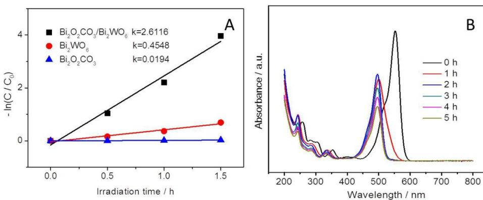
Fig. S8 (A) Plots of degradation rate of RhB over  $\text{Bi}_2\text{O}_2\text{CO}_3$ ,  $\text{Bi}_2\text{WO}_6$  and  $\text{Bi}_2\text{O}_2\text{CO}_3/\text{Bi}_2\text{WO}_6$  under visible light irradiation ( $k$  is the apparent rate constant,  $\text{h}^{-1}$ ). (B) Absorption spectra change of the RhB solution during the photocatalytic reaction.
