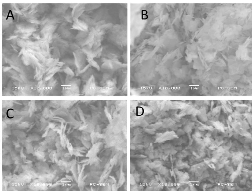
Fig. S10 SEM images of the  $\text{Bi}_2\text{O}_2\text{CO}_3/\text{Bi}_2\text{WO}_6$  composites attained after reaction for (A) 8 h, (B) 12 h, (C) 16 h, and (D) 20 h.
