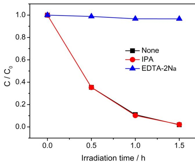
Fig. S13 Plots of Photogenerated carries trapping in the system of photocatalytic degradation of RhB over  $\text{Bi}_2\text{O}_2\text{CO}_3/\text{Bi}_2\text{WO}_6$  under visible light irradiation.
