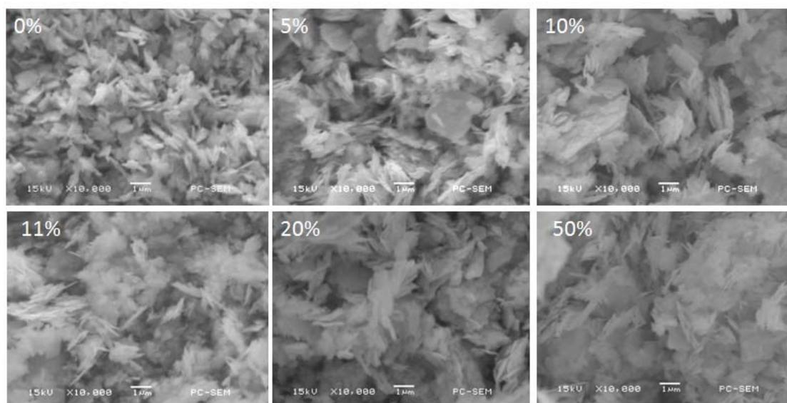
Fig. S7 SEM images of the  $\text{Bi}_2\text{O}_2\text{CO}_3/\text{Bi}_2\text{WO}_6$  composites prepared using different amounts of  $\text{g-C}_3\text{N}_4$ .
