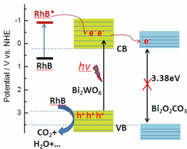
Fig. S12 Schematic diagram for the energy band structure of the  $\text{Bi}_2\text{O}_2\text{CO}_3/\text{Bi}_2\text{WO}_6$  and the possible charge transfer process under visible light irradiation.
