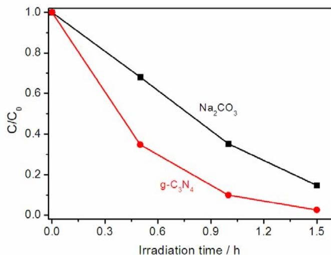
Fig. S9 Plots of degradation of RhB over  $\text{Bi}_2\text{O}_2\text{CO}_3/\text{Bi}_2\text{WO}_6$  obtained using  $\text{Na}_2\text{CO}_3$  or  $\text{g-C}_3\text{N}_4$  as the source of  $\text{CO}_3^{2-}$  under visible light irradiation. In the direct hydrothermal process, the molar ratio of the starting materials is 1:0.5:0.04 ( $\text{Bi}(\text{NO}_3)_3 \cdot 5\text{H}_2\text{O} : \text{Na}_2\text{WO}_4 \cdot 2\text{H}_2\text{O} : \text{Na}_2\text{CO}_3$ ).
