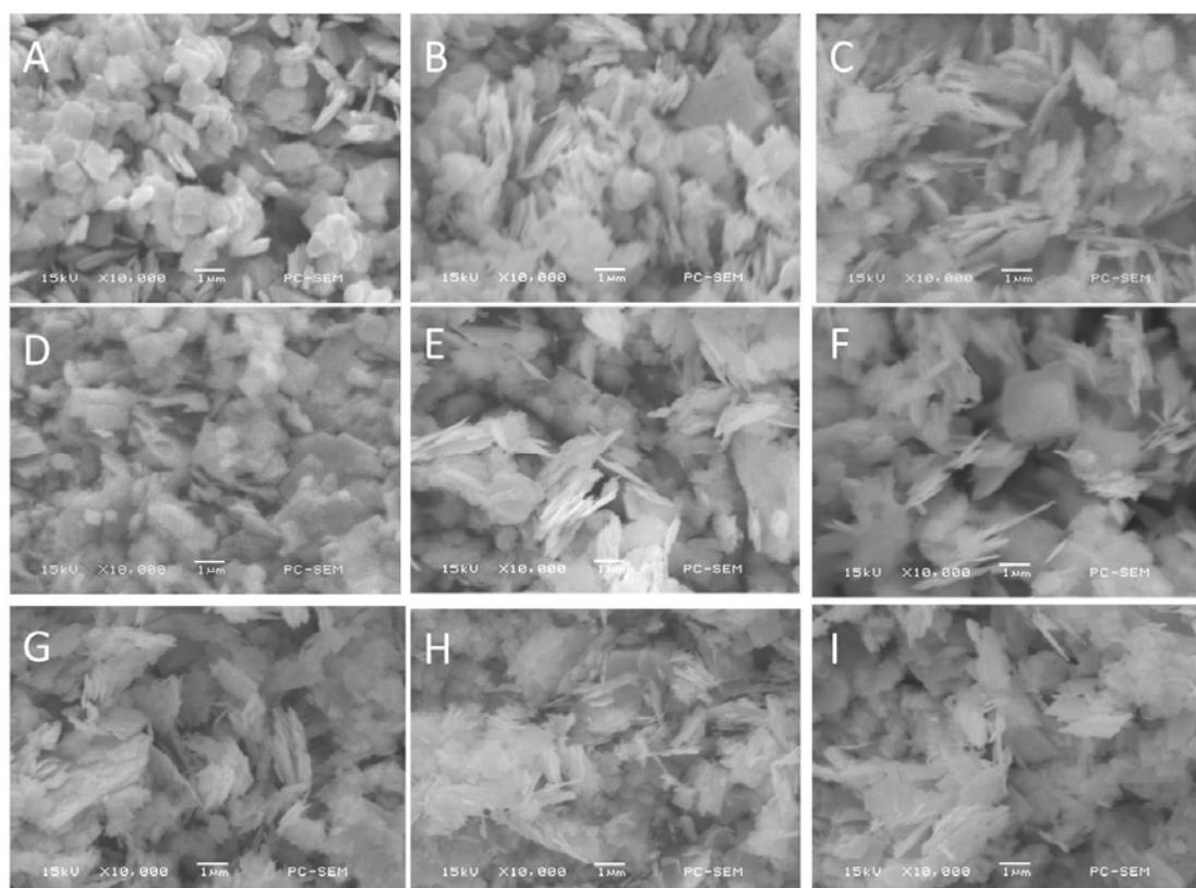
Fig. S5 SEM images of the samples prepared with different volume of NaOH, (A) 5.0 mL, (B) 6.0 mL, (C) 7.0 mL, (D) 8.0 mL, (E) 6.4 mL, (F) 6.5 mL, (G) 6.6 mL, (H) 6.7 mL, and (I) 6.8 mL.
