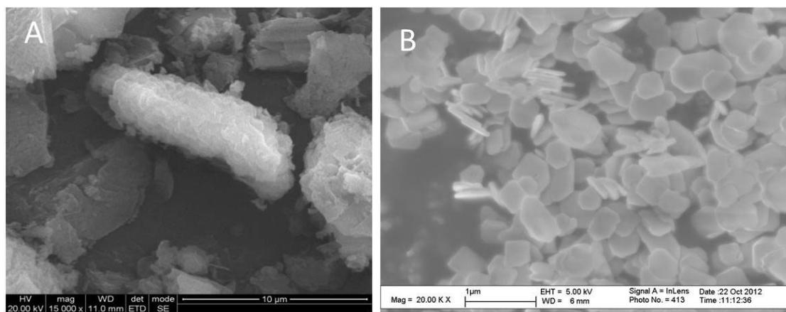
Fig. S1 SEM images of g-C<sub>3</sub>N<sub>4</sub> (A) and Bi<sub>2</sub>O<sub>2</sub>CO<sub>3</sub> (B).
