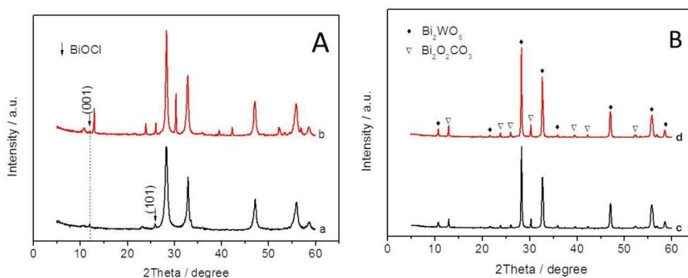
Fig. S4 XRD patterns of the samples prepared with different volume of NaOH, (a) 5.0 mL, (b) 6.0 mL, (c) 7.0 mL, and (d) 8.0 mL.
