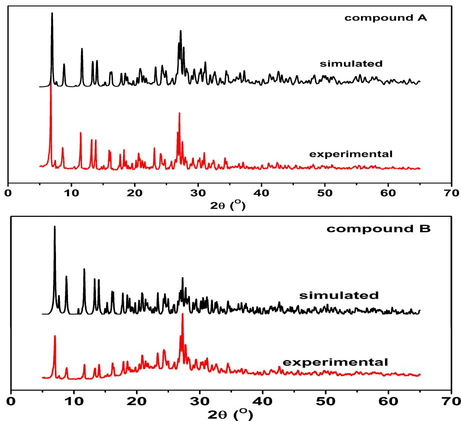
**Figure S5** PXRD of compound **A** and its corresponding dehydrated phase **B** at room temperature. The phase purity for **A** and **B** was examined. Calculated pattern from the single crystal structure of **A** and **B** (black); observed from an as-synthesized sample of **A** and **B** (red).
