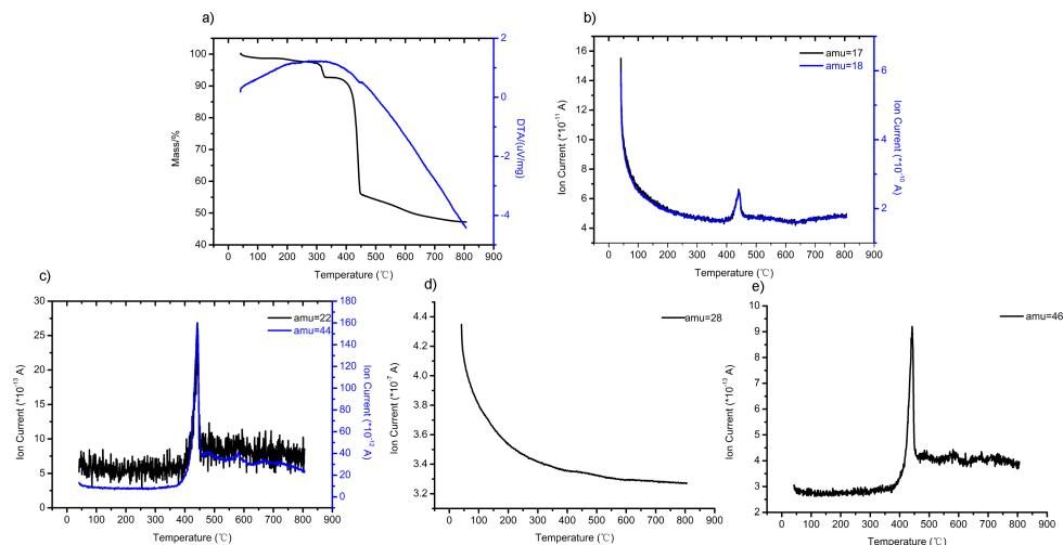
**Figure S7** a) TG and DTA curve of A that is heat treated at 100  $^{\circ}\text{C}$  (A has converted to the dehydrated phase B). b), c), d), e) The Mass Spectrometer of the detected gas.
