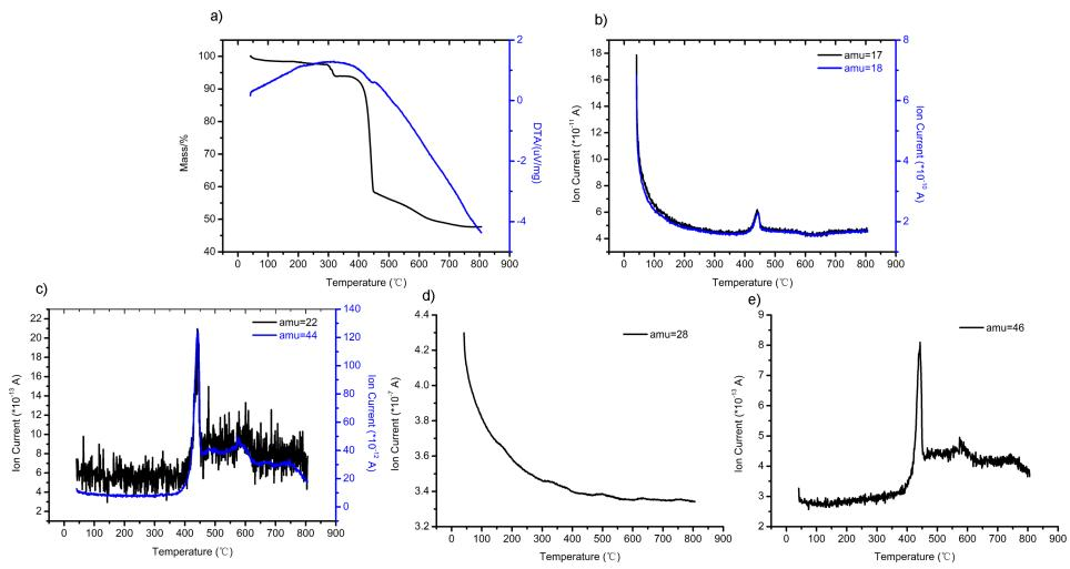
**Figure S8** a) TG and DTA curve of **A** that is heat treated at 220 °C (**A** has converted to the dehydrated phase **B**). b), c), d), e) The Mass Spectrometer of the detected gas.
