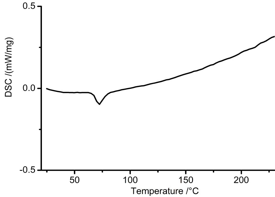
**Figure S9** DSC of **A** measured in the range from 25 to 230 °C under a nitrogen atmosphere with a heating rate of 5 °C per minute. At 62 °C, **A** starts to lose guest water molecules accompanied with the heat release behavior.
