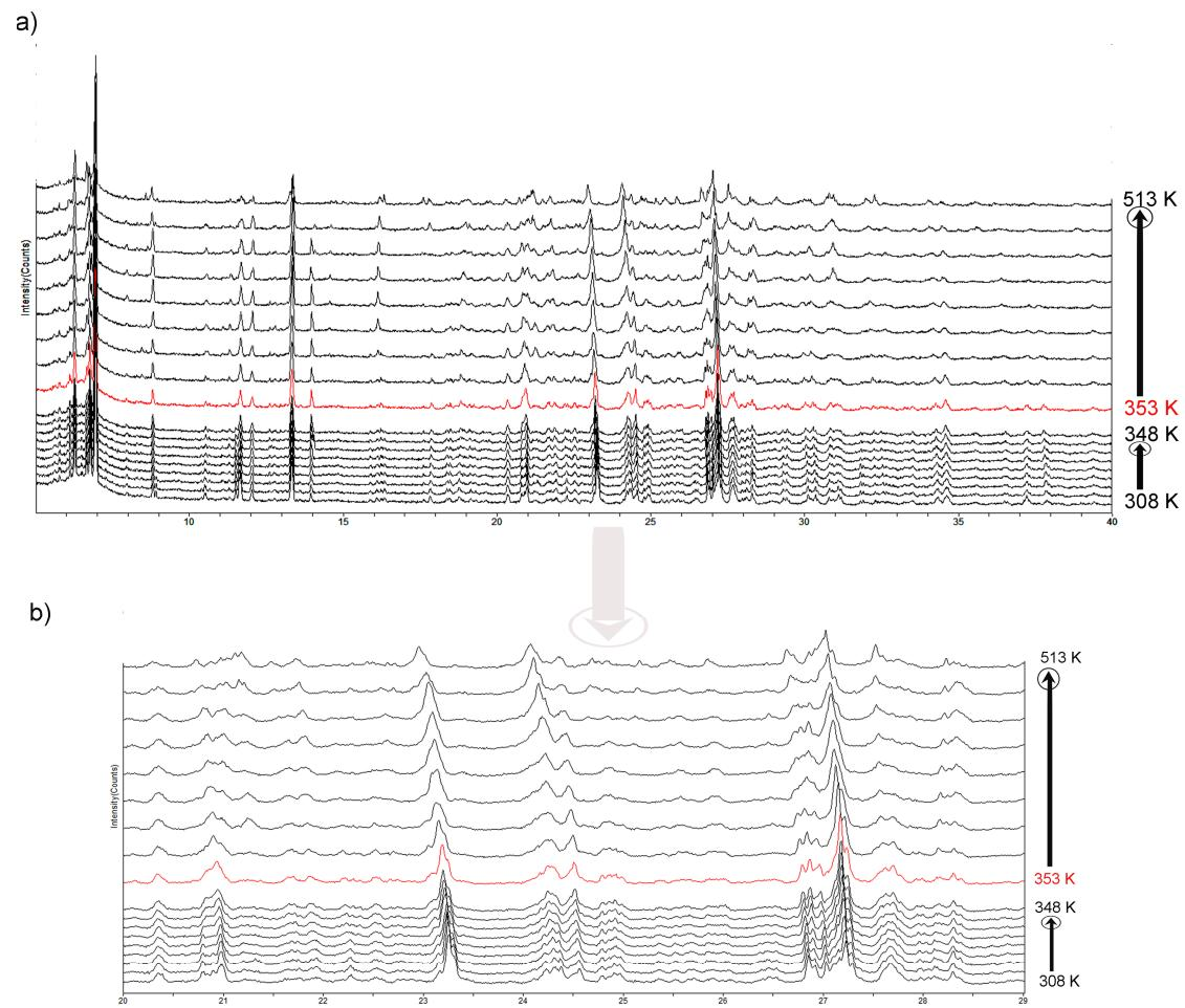
**Figure S4** Uncorrected VT-PXRD patterns of **A** recorded from 308 K to 348 K with a step size of 5 K, then from 353 K to 513 K ( $\Delta T/\text{step} = 20 \text{ K}$ ) ( **A** has converted to the dehydrated phase **B** at 353 K). b) is part of a).
