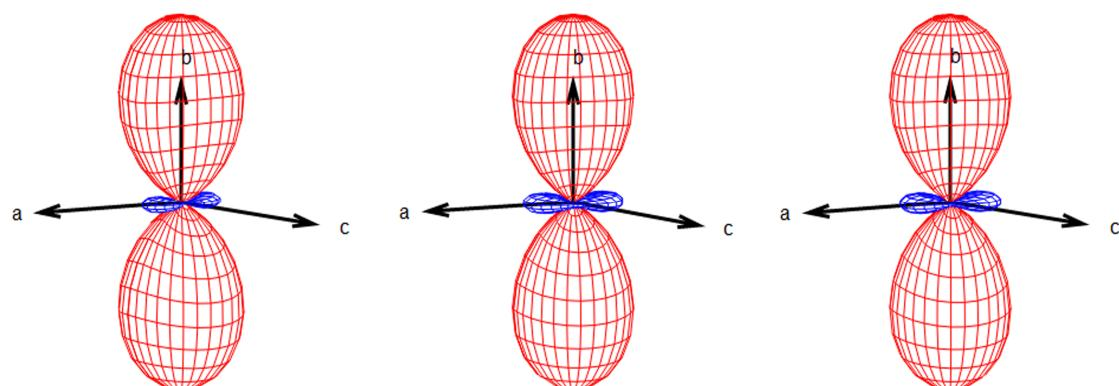
**Figure S1** The expansivity indicatrix of **A** (100-340 K) (left), **B** (100-340 K) (middle), **B** (100-500 K) (right) relating the principal axes of thermal expansion (red = positive; blue = negative thermal expansion).<sup>[5]</sup>
