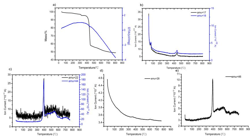
**Figure S6** a) TG and DTA curve of A at room temperature. b), c), d), e) The Mass Spectrometer of the detected gas.
