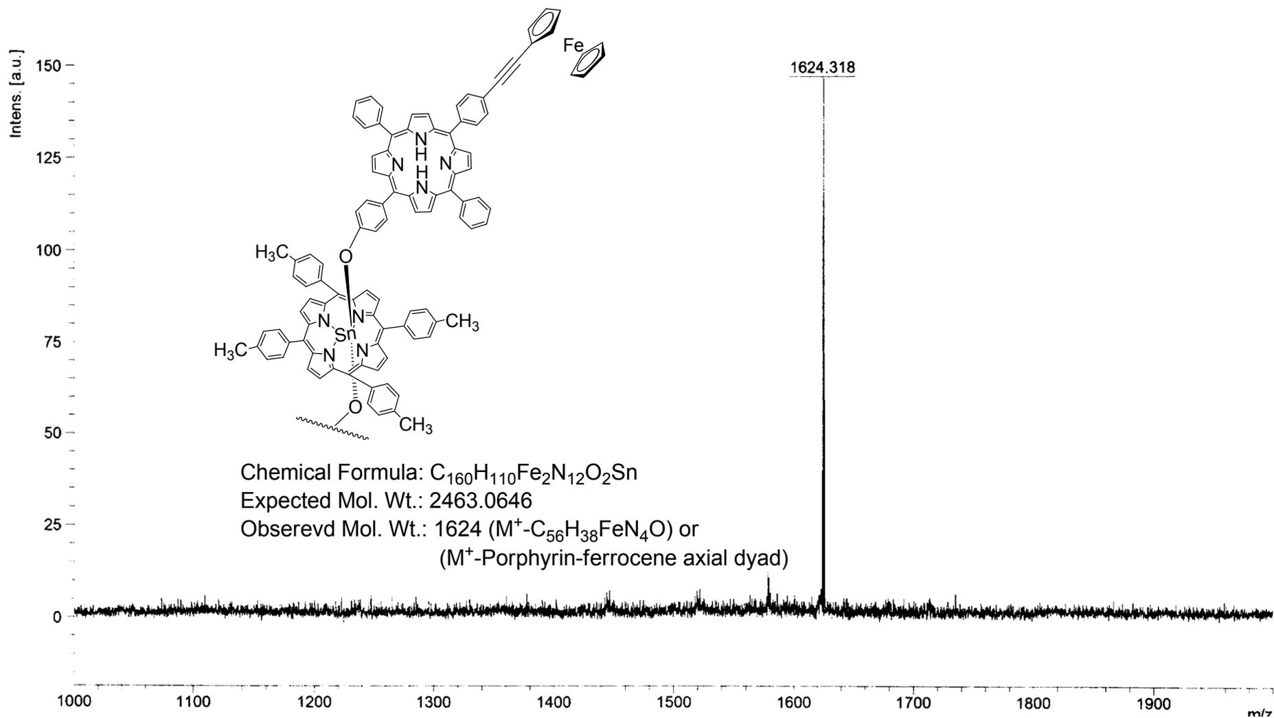
Figure S7: MALDI-TOF spectrum of pentad 1
