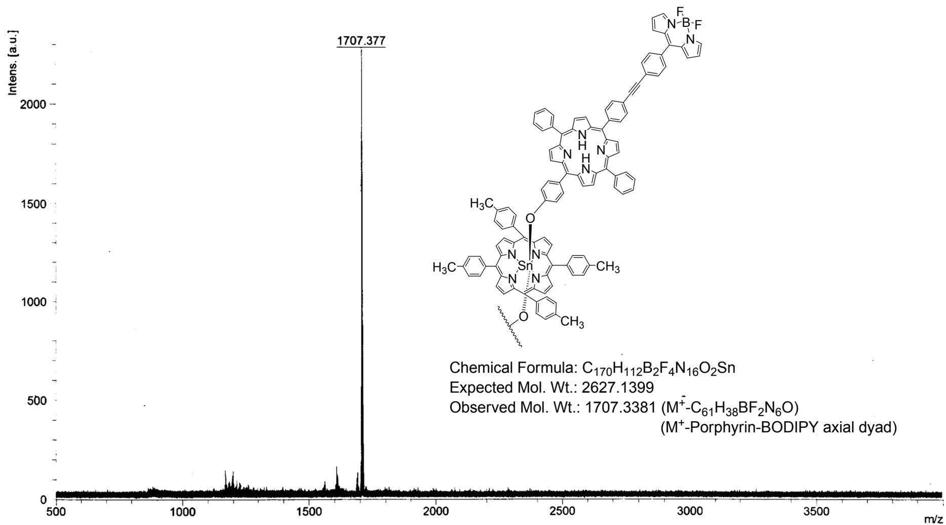
Figure S8: MALDI-TOF spectrum of pentad 2
