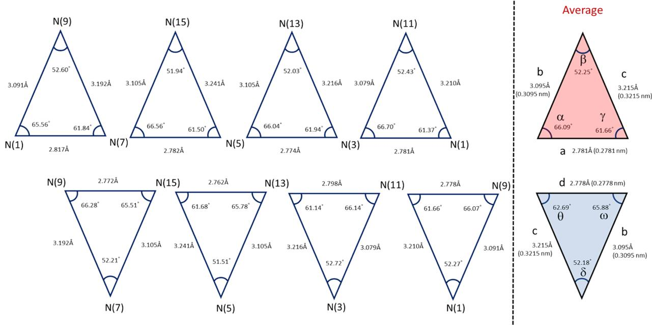
**Figure S3-4.** Schematic illustration (distance and angles) of the square-antiprismatic coordination site in the multiple-decker Dy(III)-Pc systems: DyPc<sub>2</sub>.
