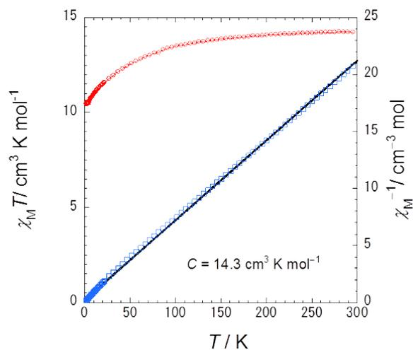
**Figure S4.** Temperature ( $T$ ) dependence of  $\chi_M T$  and  $\chi_M^{-1}$  for powder samples of **1** in a field of 1000 Oe. In the  $\chi_M^{-1}$  versus  $T$  plot, the black solid line represents a linear fit of all data.
