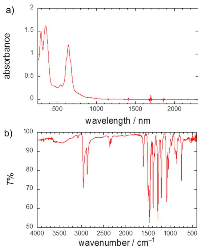
**Figure S1.** a) Electronic spectra of **1** in  $\text{CHCl}_3$  ( $\sim 10^{-5}$  M) at 298 K. b) FT-IR spectra of **1** as KBr pellets at 298 K.
