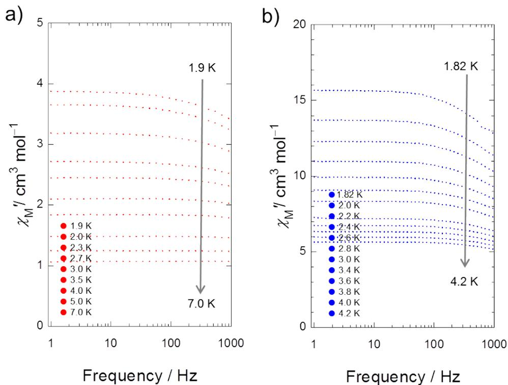
**Figure S6.** Temperature ( $T$ ) and frequency ( $\nu$ ) dependent of the ac measurements ( $\chi_M''$  versus  $\nu$  plots) of **1** and **2** in a zero dc field.
