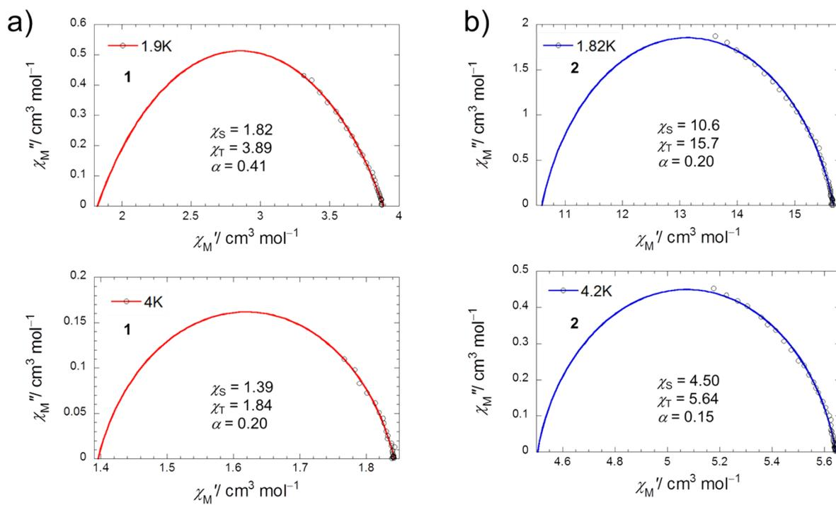
**Figure S7.** Selected Argand plots ( $\chi_M''$  versus  $\chi_M'$  plots) in a zero dc field for a) **1** and b) **2**. Solid lines (red and blue) were fitted by using a generalized Debye model (eq. 4).
