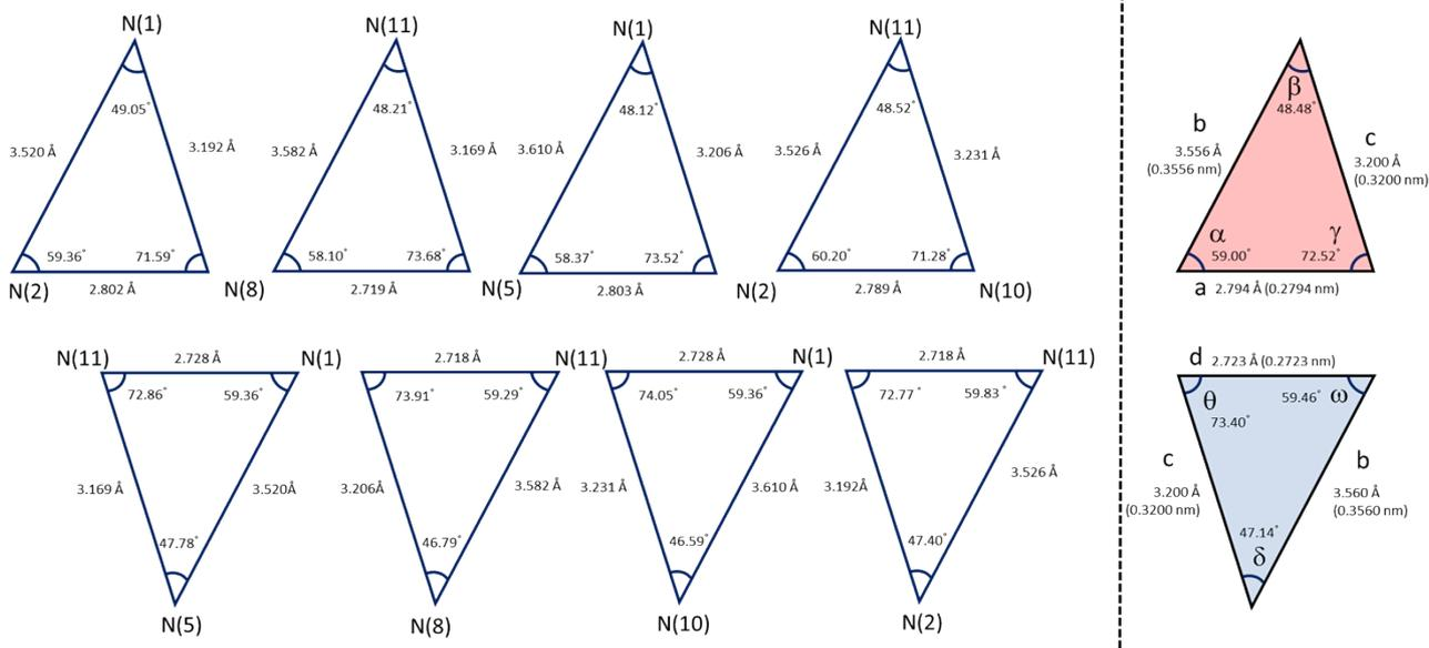
**Figure S3-1.** Schematic illustration (distance and angles) of the square-antiprismatic coordination site in the multiple-decker Dy(III)-Pc systems: DyY(obPc)<sub>3</sub> (**1**).
