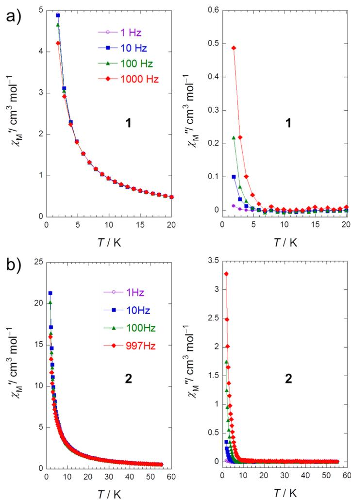
**Figure S5.** a) Frequency ( $\nu$ ) and temperature ( $T$ ) dependences of the ac magnetic susceptibility in-phase ( $\chi_M'$ ) and out-of-phase ( $\chi_M''$ ) of a) **1** and b) **2** at zero dc field.
