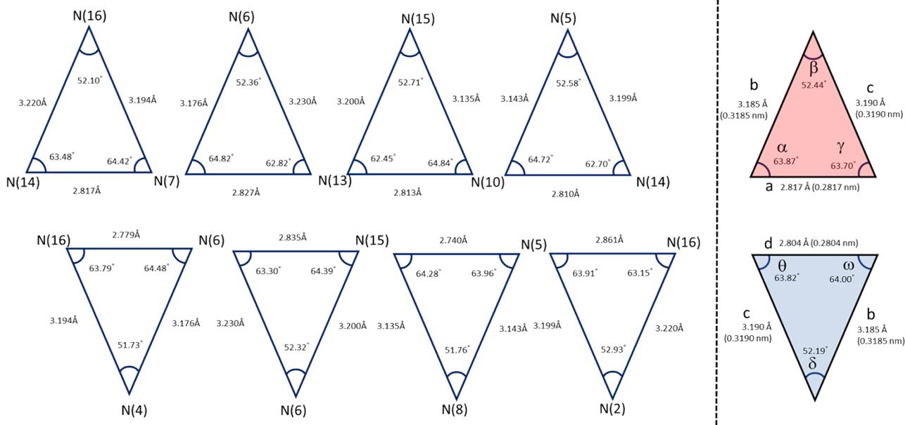
**Figure S3-3.** Schematic illustration (distance and angles) of the square-antiprismatic coordination site in the multiple-decker Dy(III)-Pc systems: Dy(obPc)<sub>2</sub>.
