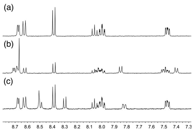
Fig. S2. Aromatic regions of the  $^1\text{H}$  NMR spectra (400 MHz,  $\text{CD}_3\text{OD}$ ) of (a)  $[\text{Cr}(\text{tpy})_2][\text{PF}_6]_3$ , (b)  $[\text{Cr}(\text{tpy})(4'-(4\text{-tolyl})\text{tpy})][\text{PF}_6]_3$  and (c)  $[\text{Cr}(\text{tpy})(5,5''\text{-Me}_2\text{tpy})][\text{PF}_6]_3$  each after the addition of NaOH.
