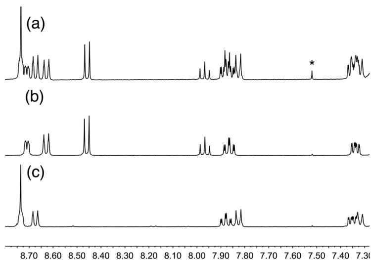
Fig. S1. Aromatic regions of the  $^1\text{H}$  NMR spectra (400 MHz,  $\text{CDCl}_3$ ) of (a) soluble material collected after filtration (see text), (b) tpy, (c) 4'-(4-tolyl)tpy. In (a), signal marked \* arises from one of the  $^{13}\text{C}$  satellite peaks of residual  $\text{CHCl}_3$ .
