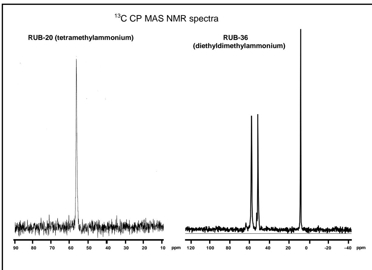
**Fig. S1:** The  $^{13}\text{C}$  CP NMR spectra of RUB-20 (left), and RUB-36 (right) are displayed here as representatives of the monoclinic and orthorhombic materials, respectively. The chemical shift values of the signals of all HLSs are listed in Table 1.
