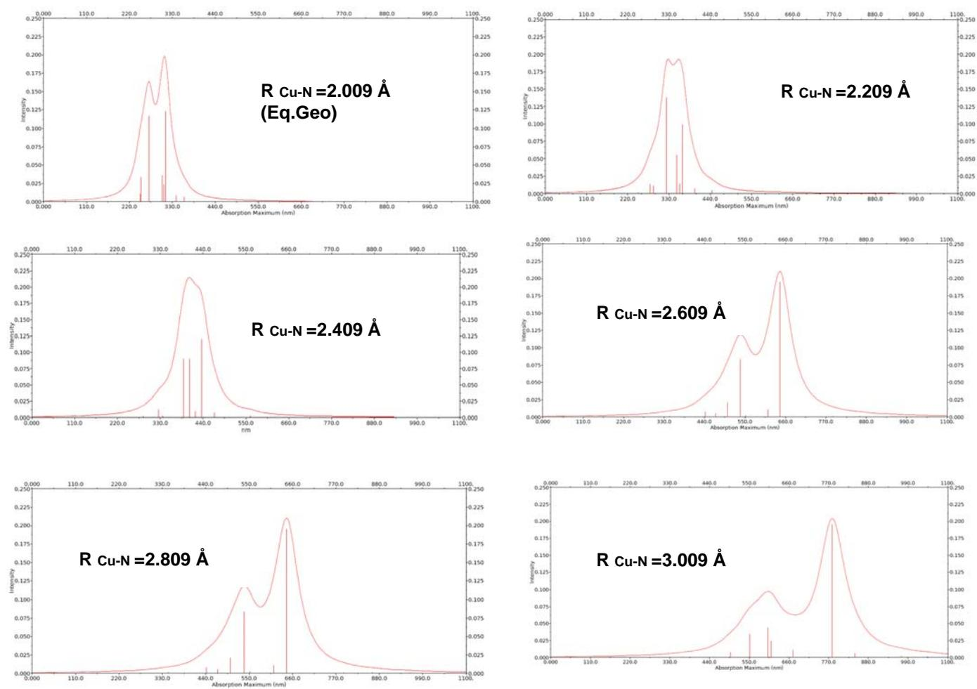
Figure S5: TD-DFT-simulated absorption spectra of the model complex  $\text{Cu}(\text{Ac})_2(\text{methylamine})_2$  complex with one water molecule.
