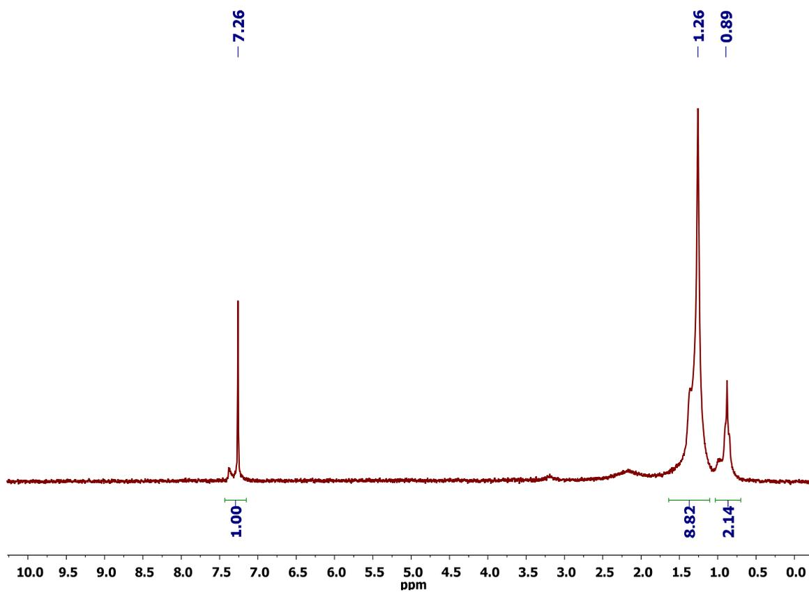
Figure S4:  $^1\text{H}$  NMR spectrum of  $\text{Cu}(\text{Ac})_2(\text{DDA})_2$  in  $\text{CDCl}_3$ .
