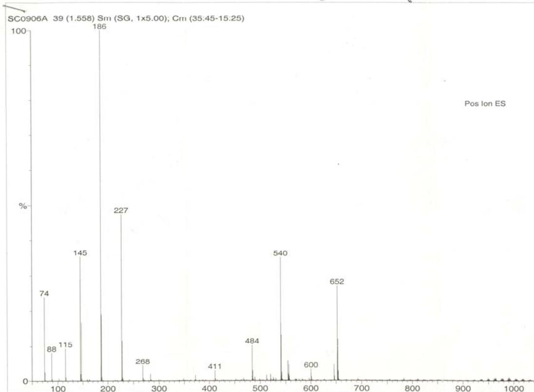
Figure S2: Mass spectrum of  $\text{Cu}(\text{St})_2(\text{DDA})_2$  compound.
