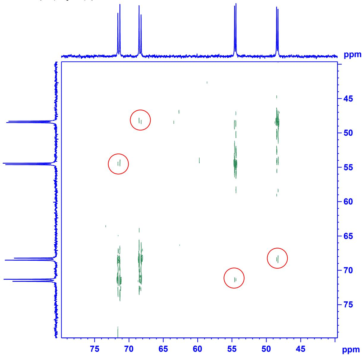
S5  $^{31}\text{P}\{\text{H}\}$  EXSY spectrum ( $\text{CD}_2\text{Cl}_2$ , 303 K) of **8** recorded with a mixing time of 250 ms indicating dynamic equilibration of all four catechol phosphine ligands.
