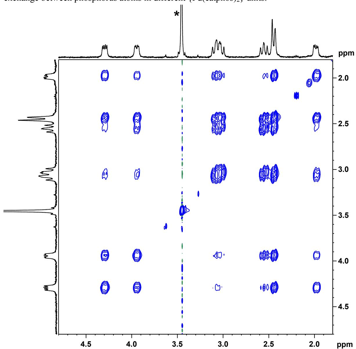
S7 Benzylic region of the  $^1\text{H}$ , $^{31}\text{P}$  HMQC spectrum of **8** ( $\text{CD}_2\text{Cl}_2$ , 273 K) enabling the assignment of benzylic protons to the ligands in different  $\{\text{Pd}(\text{catphos})_2\}$  units.
