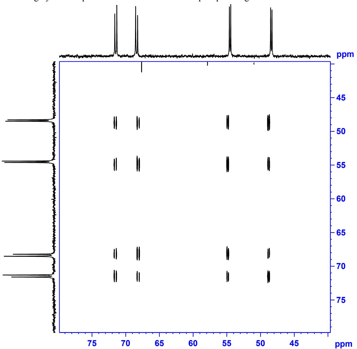
S6  $^1\text{H}$  EXSY spectrum ( $\text{CD}_2\text{Cl}_2$ , 303 K) of **8** recorded with a mixing time of 200 ms. Stars denote the signals of co-crystallised MeOH circles highlight ross-peaks indicating pairwise exchange between phosphorus atoms in different  $\{\text{Pd}(\text{catphos})_2\}$  units.
