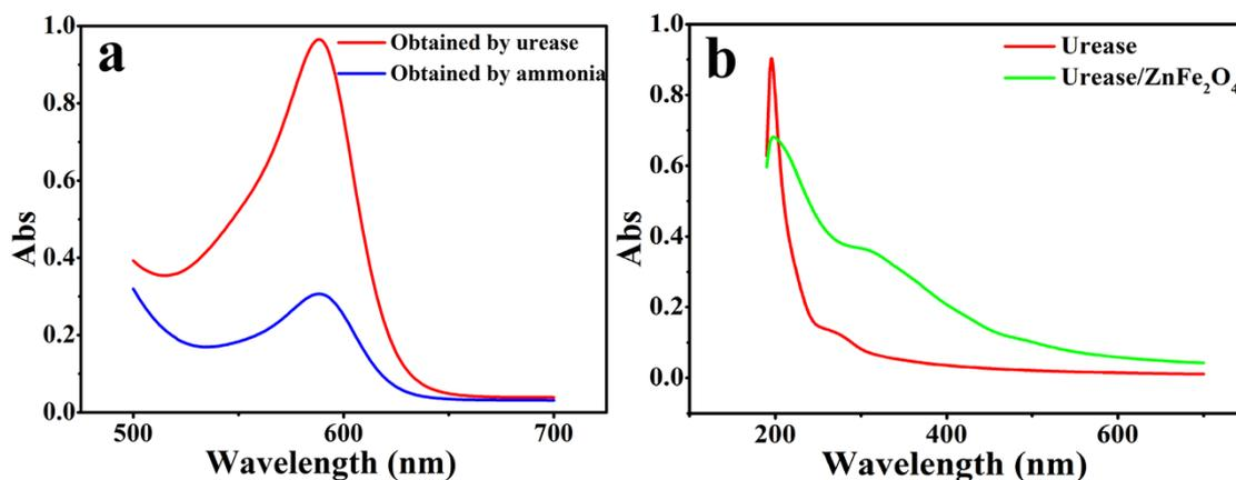
**Fig. S1 (a) UV-Vis spectrophotometer spectra of the catalytic results catalyzed by pure  $\text{ZnFe}_2\text{O}_4$  and Urease/ $\text{ZnFe}_2\text{O}_4$  nanocomposites and (b) UV-Vis spectrophotometer spectra of pure urease and Urease/ $\text{ZnFe}_2\text{O}_4$  nanocomposites.**
