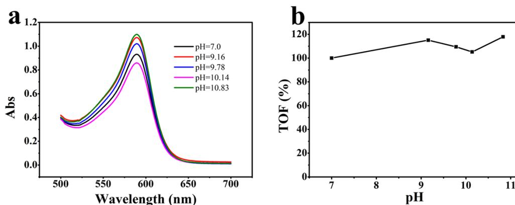
**Fig. S2 (a) UV-Vis spectrophotometer spectra of the catalytic results catalyzed by Urease/ZnFe<sub>2</sub>O<sub>4</sub> nanocomposites after bathed in different buffer solutions ranging from 7 to 11, (b) the tolerance properties to pH of Urease/ZnFe<sub>2</sub>O<sub>4</sub> nanocomposites.**
