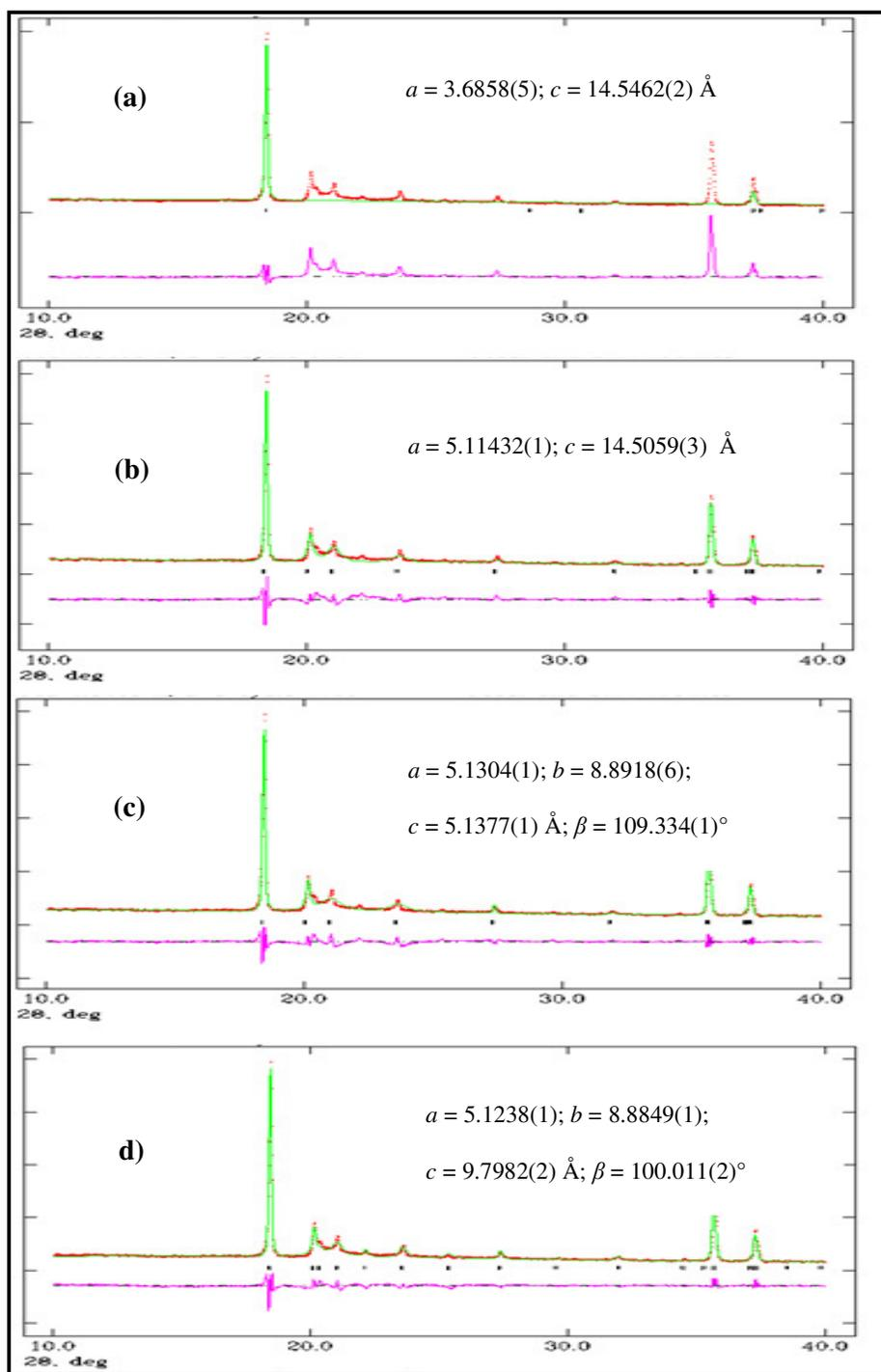
**Fig. S1.** Powder X-Ray diffraction pattern of  $\text{Li}_4\text{CrSbO}_6$  indexed using (a)  $R\text{-}3m$  subcell, (b)  $P3_1I2$  supercell, (c)  $C2/m$  supercell, and (d)  $C2/c$  supercell; Red line experimental data; green line calculated profile; pink line difference profile; vertical bars, Bragg positions.
