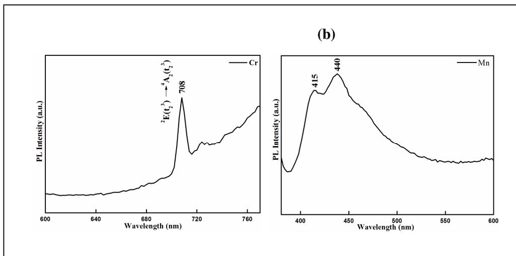
**Fig. S3** (a) Diffuse reflectance spectra of  $\text{Li}_4\text{MSbO}_6$  ( $M = \text{Cr, Mn, Fe, Al, Ga}$ ) and (b) Photoluminescence spectra of  $\text{Li}_4\text{CrSbO}_6$  and  $\text{Li}_4\text{MnSbO}_6$ .
