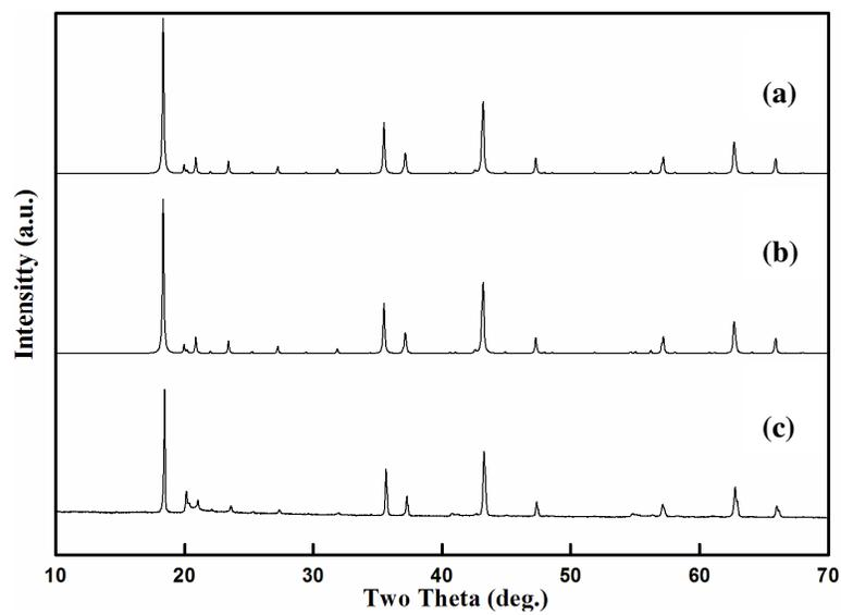
**Fig. S2** (a) PXRD plot derived from the measured SCXRD intensities for  $\text{Li}_4\text{CrSbO}_6$ ; (b) simulated PXRD pattern using the SCXRD solution of  $\text{Li}_4\text{CrSbO}_6$ ; (c) PXRD pattern obtained for the bulk polycrystalline  $\text{Li}_4\text{CrSbO}_6$ .
