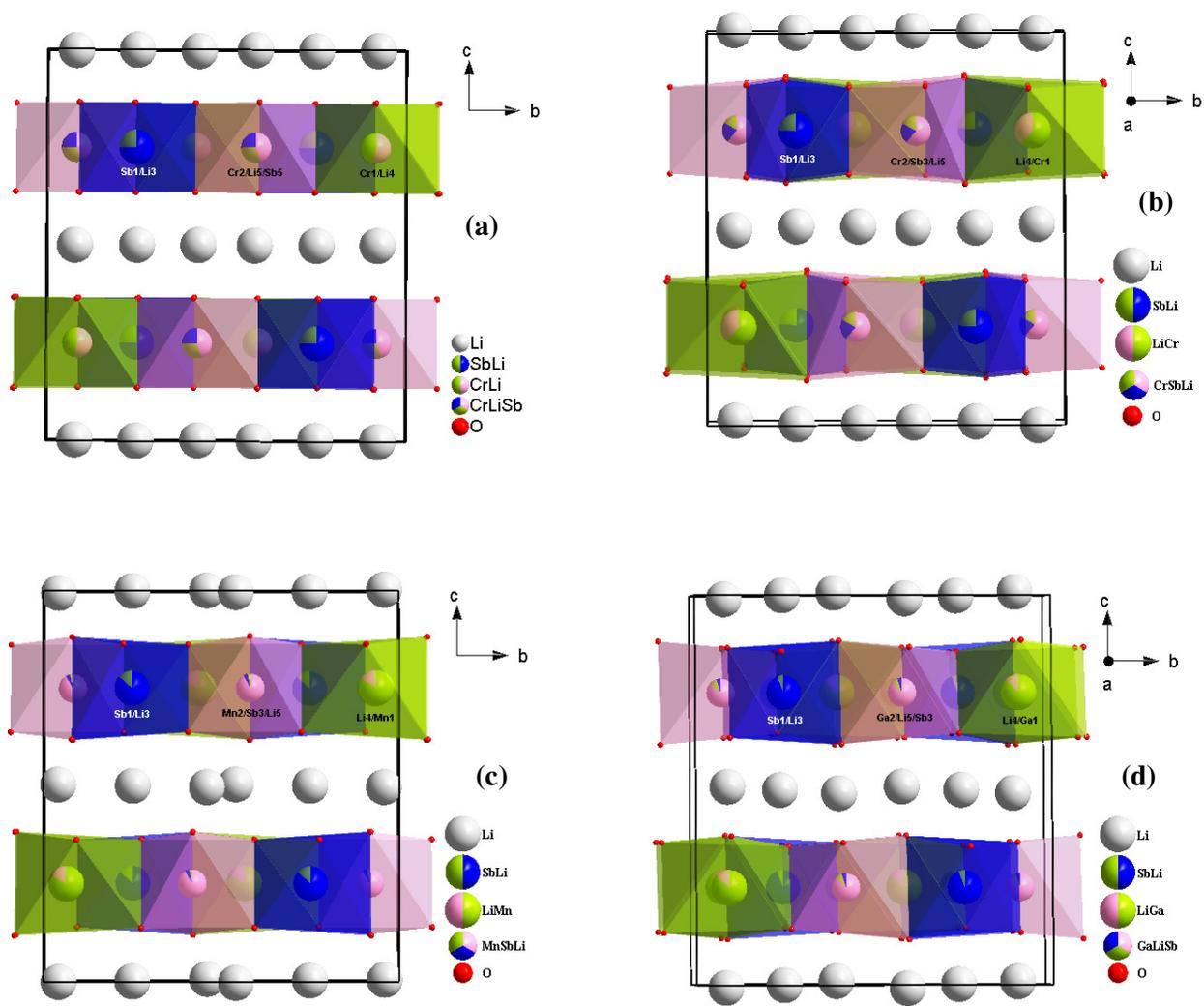
**Fig. S4** Structure of  $\text{Li}_4\text{MSbO}_6$  (M = (a) Cr (SCXRD), (b) Cr (PXR), (c) Mn, (d) Ga) perpendicular to the honeycomb layers.
