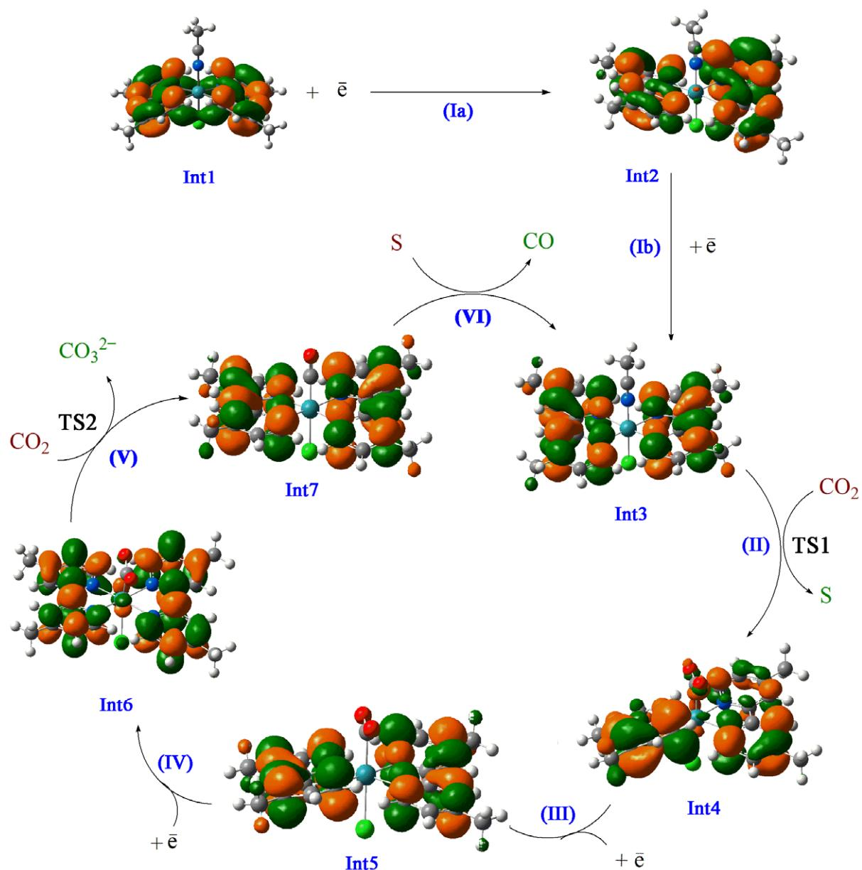
**Scheme S2** The schematic representation of LUMOs of the species in the proposed mechanism for electrocatalytic reduction of  $\text{CO}_2$  by the Ru(II) complex.
