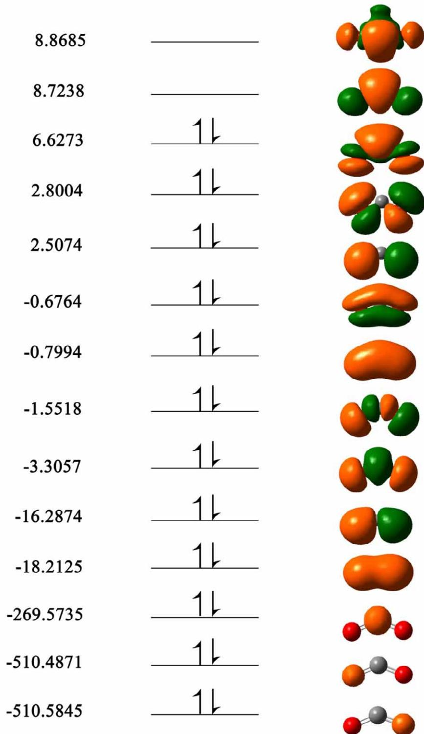
**Scheme S3** Schematic representation of the calculated molecular-orbitals in  $\text{CO}_2^{2-}$  (bent geometry) with their energy levels (eV).
