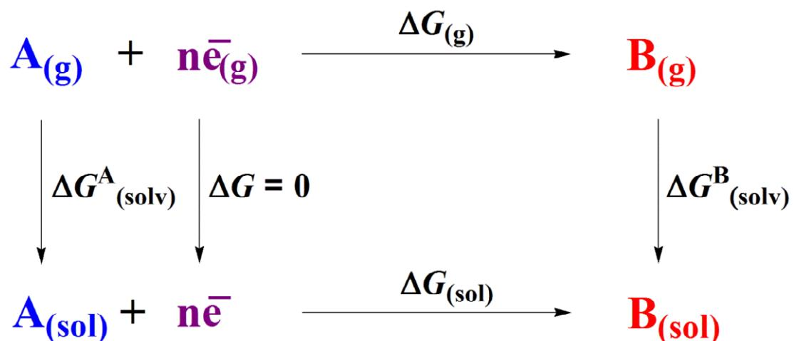
**Scheme S4** Thermodynamic cycle for a typical reaction. In the proposed catalytic cycle,  $\mathbf{n}$  can be 0 (steps **II**, **V** and **VI**) or 1 (steps **I**, **III** and **IV**). It should be mentioned that in steps **II**, **V** and **VI**, there are more than one reactant (and also one product) but the overall pattern of eqns does not change.
