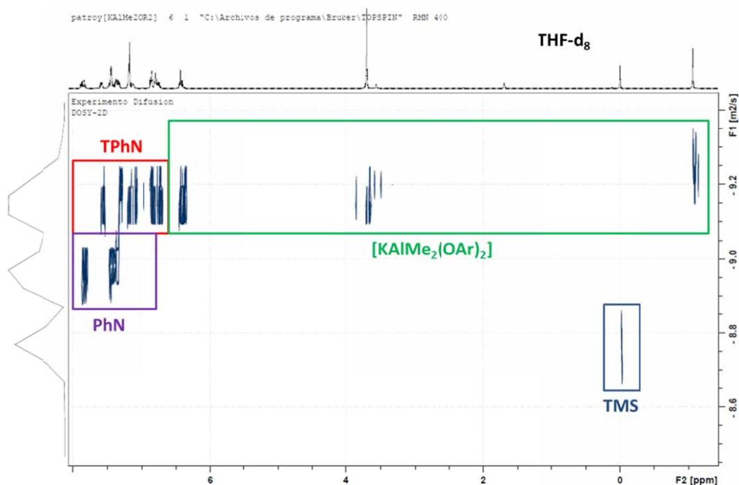
Figure S2. 2D DOSY NMR experiment of the mixture of TMS, PhN, TPhN and 3c in THF-d 8 . The x- and y-axis represent the regular ^1H chemical shift and the relative diffusion rate, respectively.
