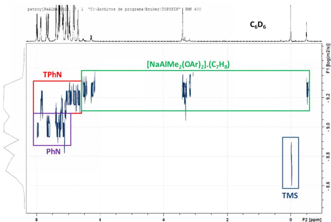
Figure S1. 2D DOSY NMR experiment of the mixture of TMS, PhN, TPhN and 3b in C_6D_6 . The x- and y-axis represent the regular ^1H chemical shift and the relative diffusion rate, respectively.
