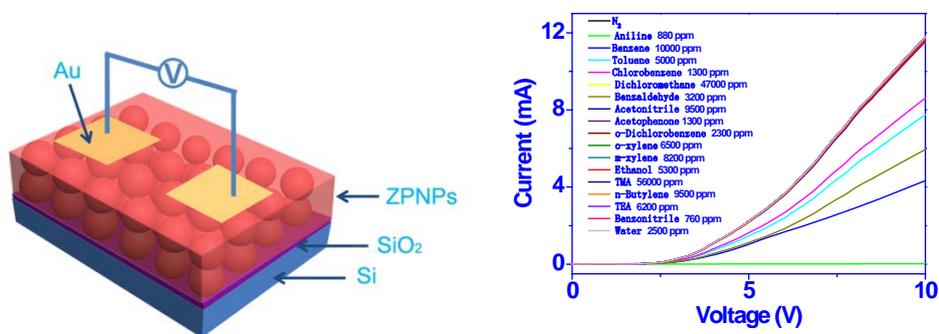
**Figure S4.** (a) schematic model of the ZPNPs film sensor; (b) Current-voltage curves of the sensor in nitrogen and when exposed to a series of VOCs and water vapor.
