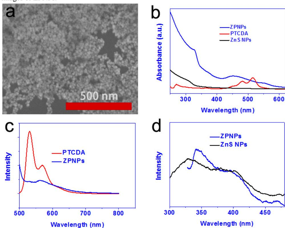
**Figure S2.**(a) SEM image of the ZPNPs. b) UV-vis absorption spectrum of ZPNPs and ZnS NPs in ethanol, PTCDA in DMF solution; (c) fluorescence emission spectrum of ZPNPs in ethanol and PTCDA in DMF solution, using a 480 nm excitation; (d) fluorescence emission spectrum of ZPNPs and ZnS NPs in ethanol, using a 300 nm excitation.
