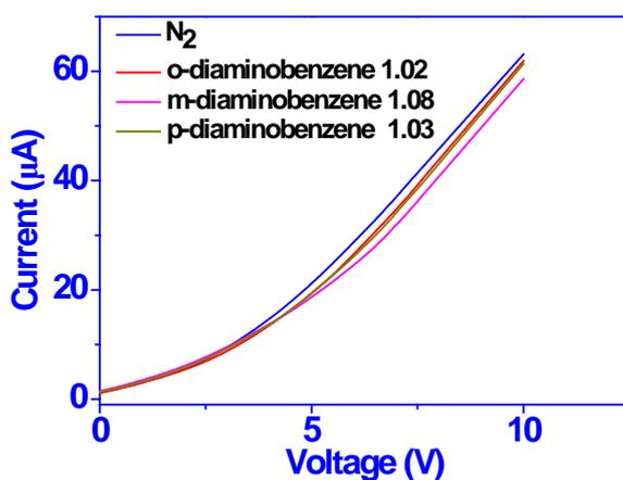
**Figure S5.** The current-voltage curve of the ZPNPs sensor before and after exposed to phenylenediamines.
