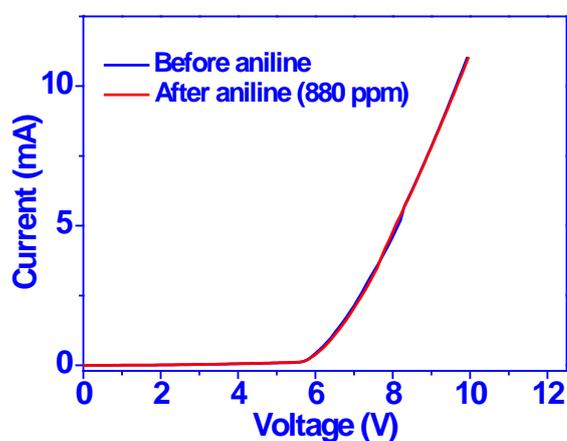
**Figure S7.** Current-voltage curve of the ZnS NP film sensor before and after exposed to aniline (880 ppm).
