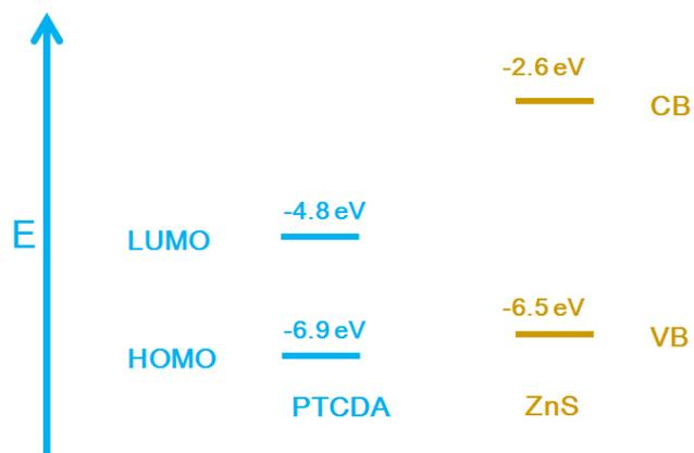
**Figure S9** Energy level alignments of PTCDA and ZnS relative to vacuum level.<sup>39, 40</sup>
