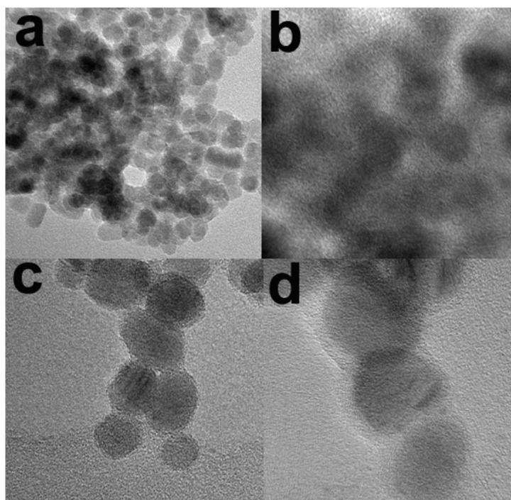
**Figure S1** (a) TEM and (b) HRTEM images of PZn nanoparticles, (c) and (d) high-magnification TEM images of ZPNPs.
