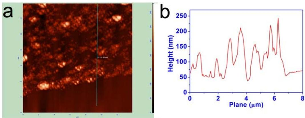
**Figure S3.** (a) AFM image of the ZPNPs film; (b) height map the film along the marked line in (a).
