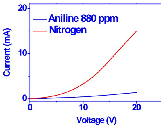
**Figure S8.** Current-voltage curve of the PTCDA film sensor before and after exposed to aniline at the concentration of 880 ppm.
