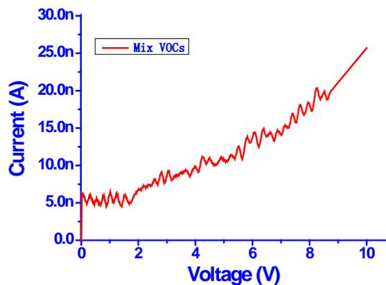
**Figure 6** The current-voltage curve of competition experiment using mix VOCs (mixed the saturated vapor of aniline, benzene, toluene, chlorobenzene, and benzaldehyde). The ZPNPs sensor exposed to mix VOCs.
